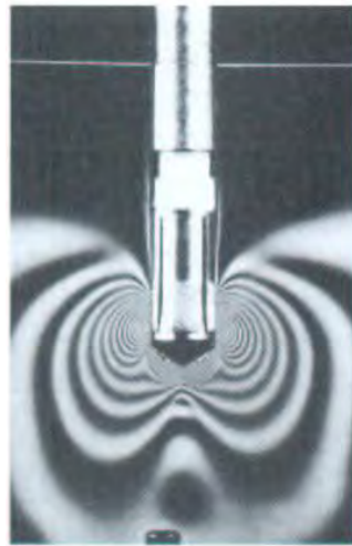
Fig. 2.22 Stress contours in the anchorage zone of a torque-controlled expansion anchor (Seghezzi (1983))
