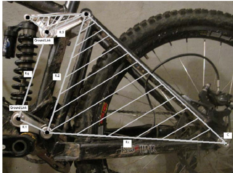
Mountain Bike Rear Suspension Mechanism
