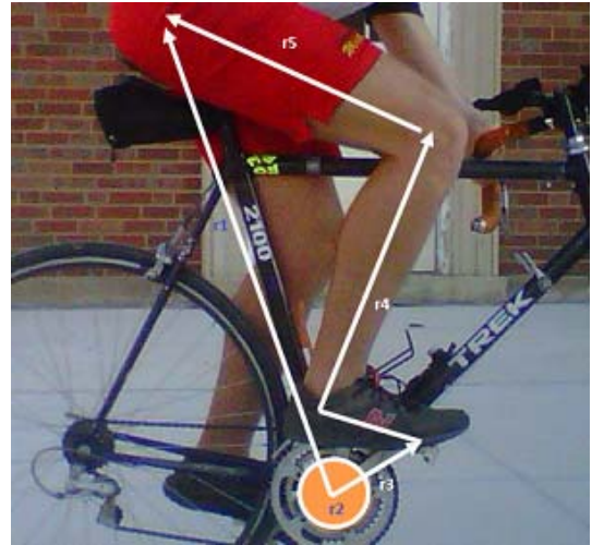
Bicycle/Human Leg 4-bar Mechanism (lock ankle)
