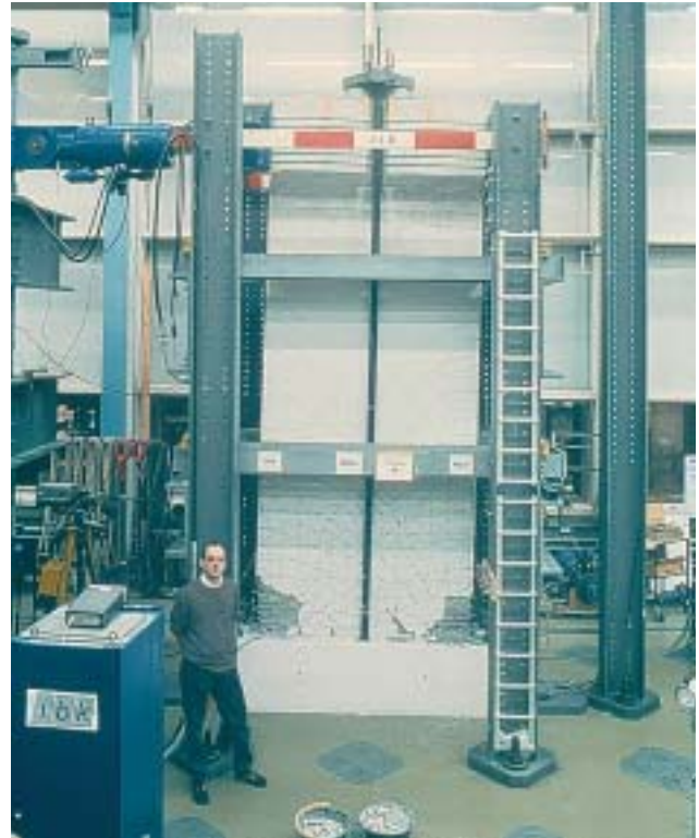
23/1 Static-cyclic tests on the lower part of 1:2 scale 6-storey reinforced concrete structural walls have clearly demonstrated the effectiveness of a ductile design [Da 99]. The capacity designed walls achieved, at little additional cost, a seismic capacity 3 to 4 times larger than that of walls conventionally designed according to the Swiss building code SIA 162.
