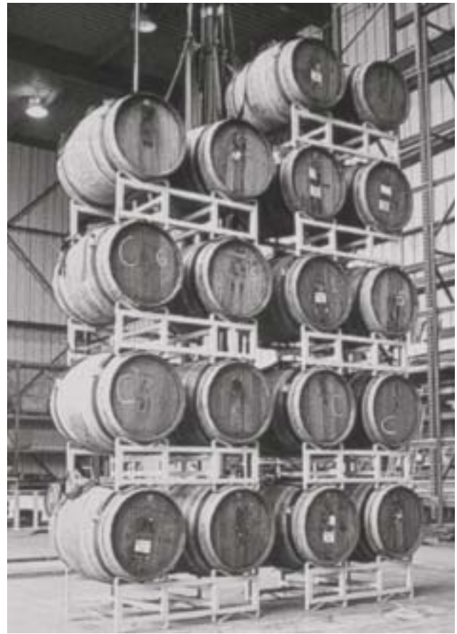
35/9 And even storage frames for wine barrels can be tested on an earthquake simulator (shaking table)... (Berkeley 2000).
