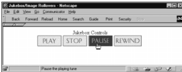
Figure 12-1: Typical mouse rollover image swapping
