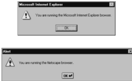
Figure 16-10: Results of the alert() method in Listing 16-20 in Internet Explorer 5 and Navigator 6 for Windows 98
