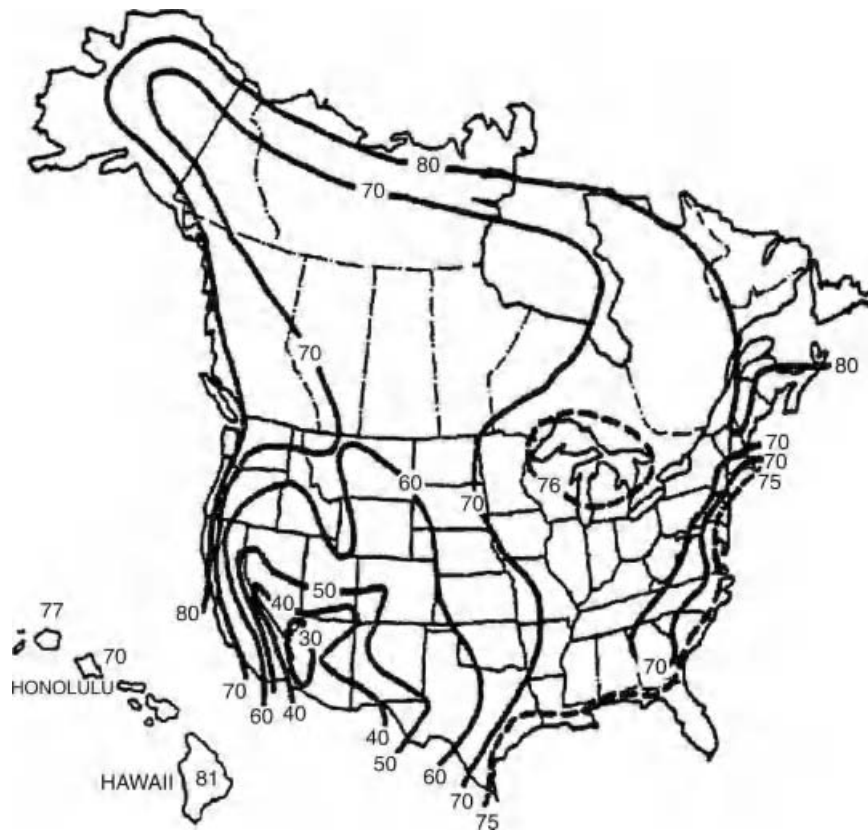
Fig. 13.10 Annual average ambient relative humidity in percent [AASHTO Fig. 5.4.2.3.3-1]. [From AASHTO LRFD Bridge Design Specifications . Copyright © 2010 by the American Association of State Highway and Transportation Officials, Washington, DC. Used by permission.]
