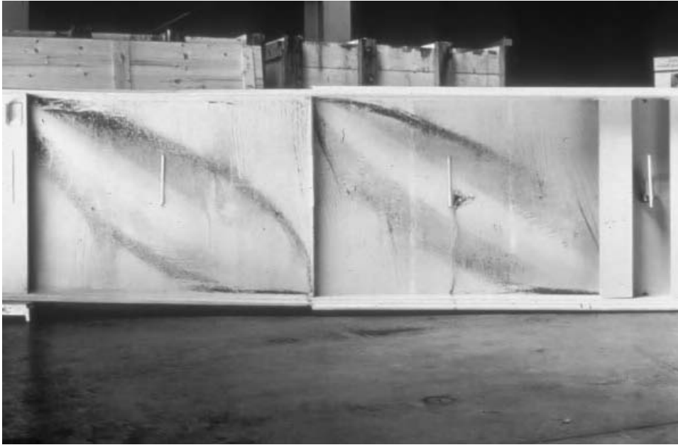
Fig. 19.50 Thin-web girder after testing. (Photo courtesy of John Fisher, ATLSS Engineering Research Center, Lehigh University.)
