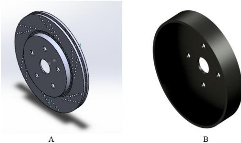
Figure 3 :(A) ventilated disc, (B) drum disc
