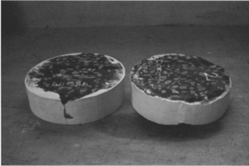
Fig. 5.6 Result of wheel-tracking cores with modified (left) and unmodified (right)
