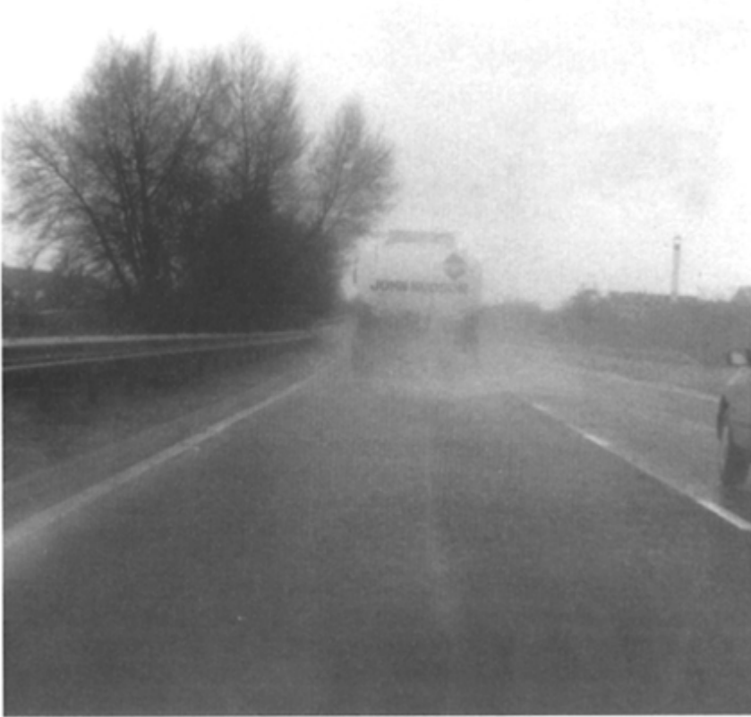
Fig. 7.8 Spray generated by a tanker travelling on rolled asphalt
