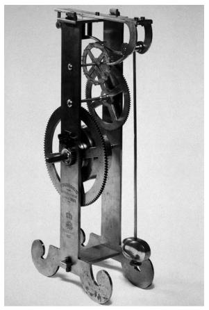
Based on a discovery by Galileo, this clock mechanism uses a pendulum to regulate its motion. (The Granger Collection)
