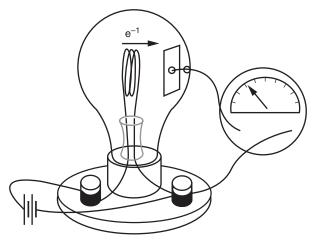
The Edison effect: Thomas Edison inserted a metal plate into a bulb and noted that when the power was turned on, a meter attached to the plate indicated that current was flowing through the air between the glowing filament and the plate.
