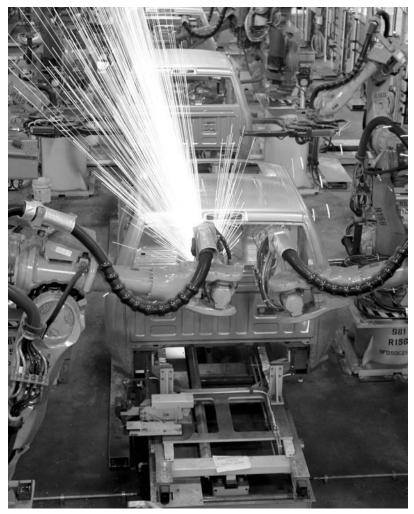
Robot welders at work on an automotive assembly line. (AP Photo/Carlos Osorio)
