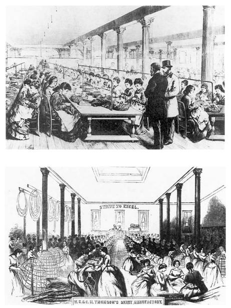
Machinery was not always a prerequisite for factory production. Note the similarity in the general layout of two clothing factories, one operating before the invention of the sewing machine, the other afterward. (Everett Collection/Superstock; The Granger Collection, New York)
