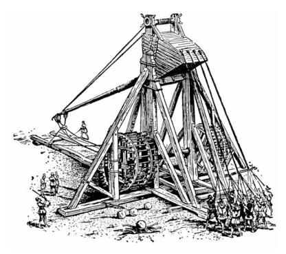
The medieval trebuchet used a counterweight and some human assistance to hurl a projectile placed at the end of the long lever arm. (The Granger Collection, New York)
