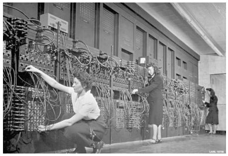
ENIAC, a first-generation electronic digital computer, was programmed by plugging and unplugging cables. (CORBIS)
