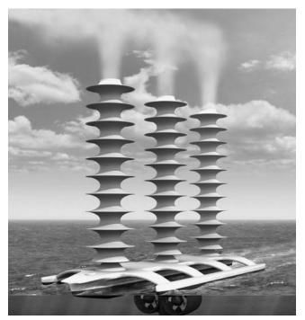
The development of technological fixes to prevent or mitigate climate change is known as geoengineering. One example is a proposed fleet of wind-powered vessels that would generate clouds of seawater droplets, which in turn would block some of the sunlight that is the source of the greenhouse effect. (John MacNeill Illustration)
