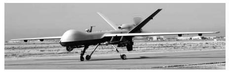
An MQ-9 Reaper landing after a mission in Iraq. A widely used drone, the Reaper is 36 ft. long with a wingspan of 66 ft. It can carry 3,800 lbs. of reconnaissance gear or 14 Hellfire air-to-ground missiles. (U.S.Air Force photo/Tech. Sgt. Erik Gudmundson)
