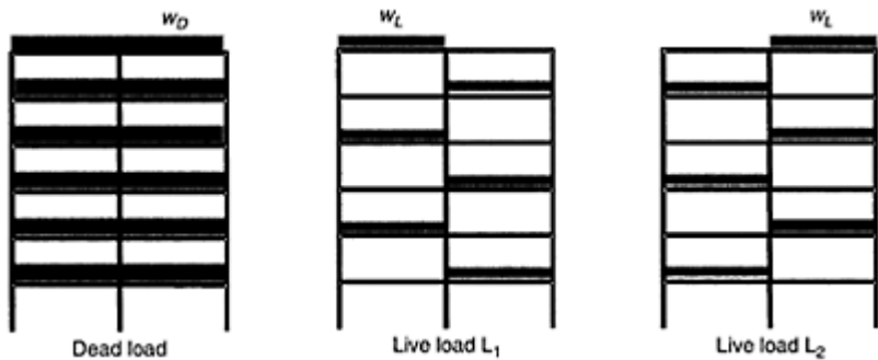
FIGURE 14.14 Distributed gravity (dead and live) loads acting on the girders of the frame.
