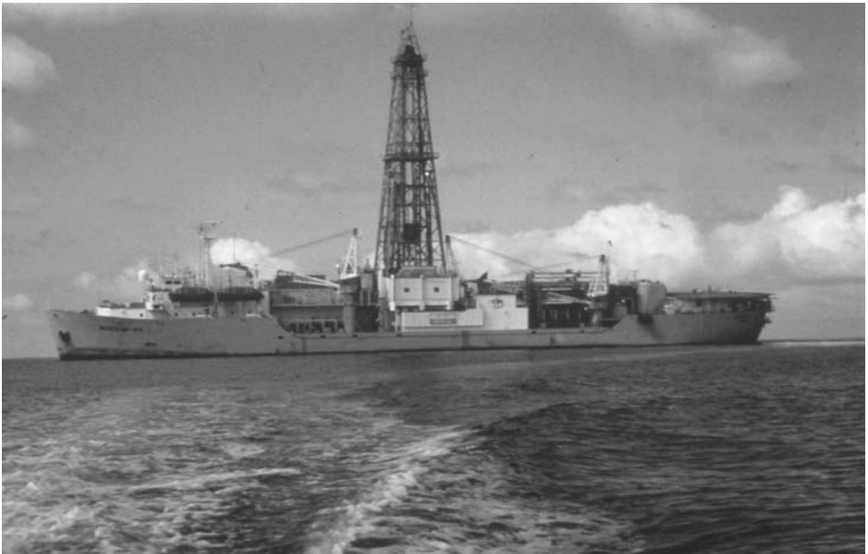
Figure 1.3 The Joides Resolution, a specially commissioned ocean-going drilling ship for coring deep-sea sediments (photo Bill Austin)
