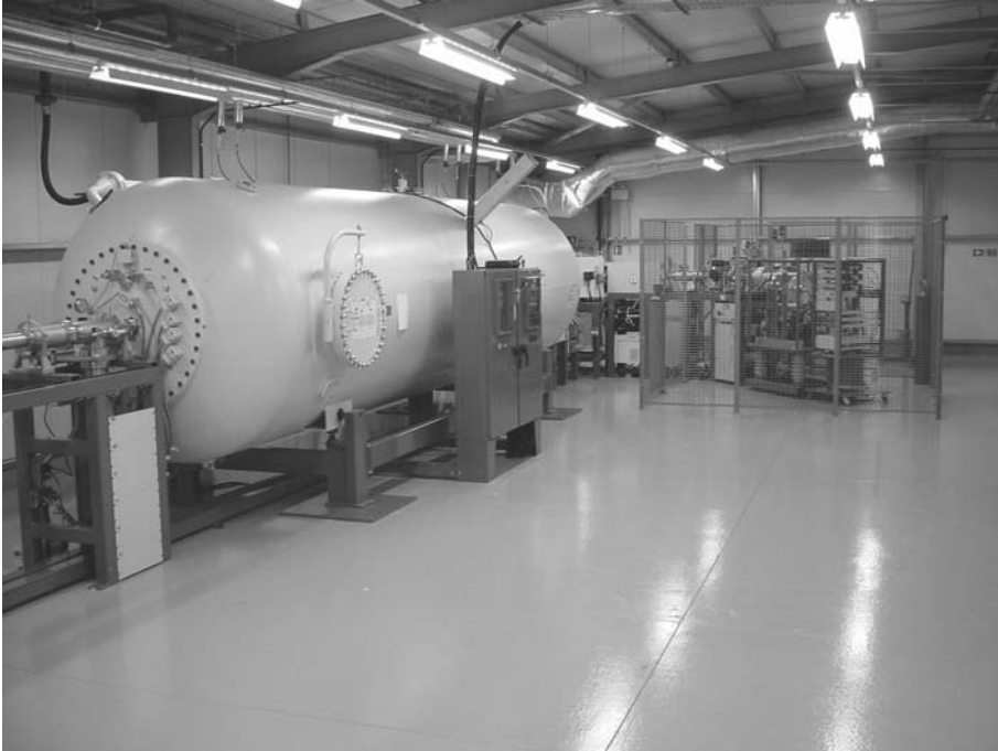
Figure 2.2 The 5-Mv National Electrostatics Corporation Accelerator Mass Spectrometer at the Scottish Universities Environmental Research Centre, East Kilbride, Scotland, UK. The accelerator itself is on the left of the photograph, while the ion source (Figure 2.4) is in the screened area to the right. See also Figure 2.3 (photo: Sheng Xu)
