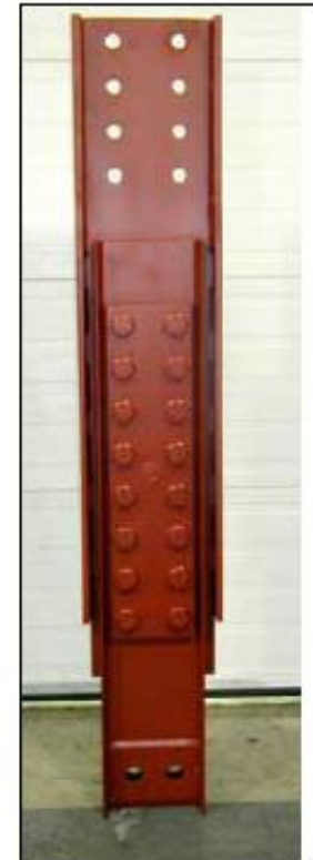
Pall Friction Damper
