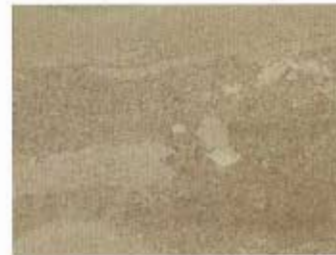
Broughton Moor slate, sanded
