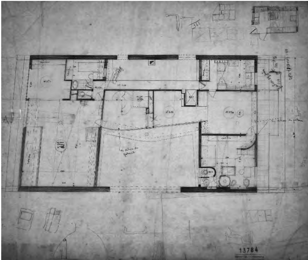
Figure 5.21 Sketch showing one of the ways Le Corbusier thought of making a transition space between the bedroom (lower right-hand side) and the dining space penthouse, 24 Rue Nungesser et Coli (1934), FLC 15653
