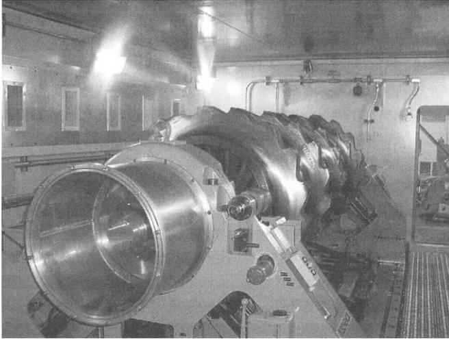
**Figure 9-4.** A large rotor in an operating speed test stand.
