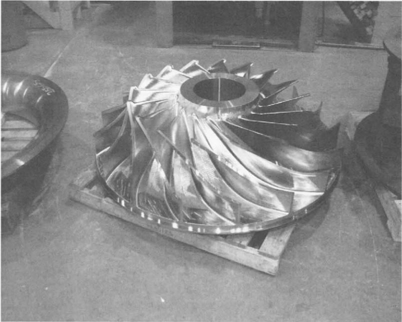
**Figure 5-35.** A centrifugal compressor impeller with machined blading performed on a five-axis milling machine. Note: The blading is integral with the impeller back plate. (Courtesy of Dresser-Rand.)
