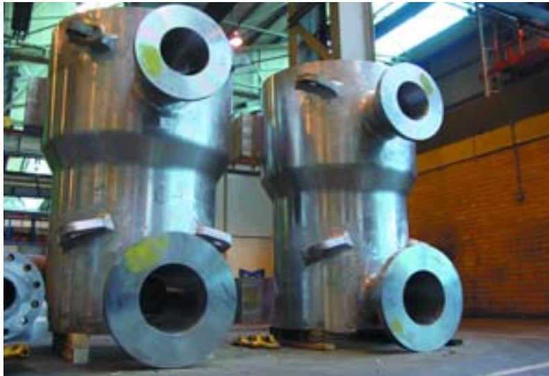
5 Forged and fully fabricated barrel casings weighing 10,000 kg each.
