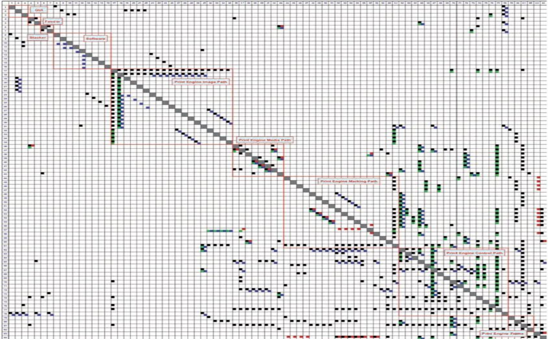
Figure 3.3.3 Product architecture DSM of the Xerox iGen3 digital printing system, indicating four types of interfaces across the 84 components, grouped into nine subsystems.
