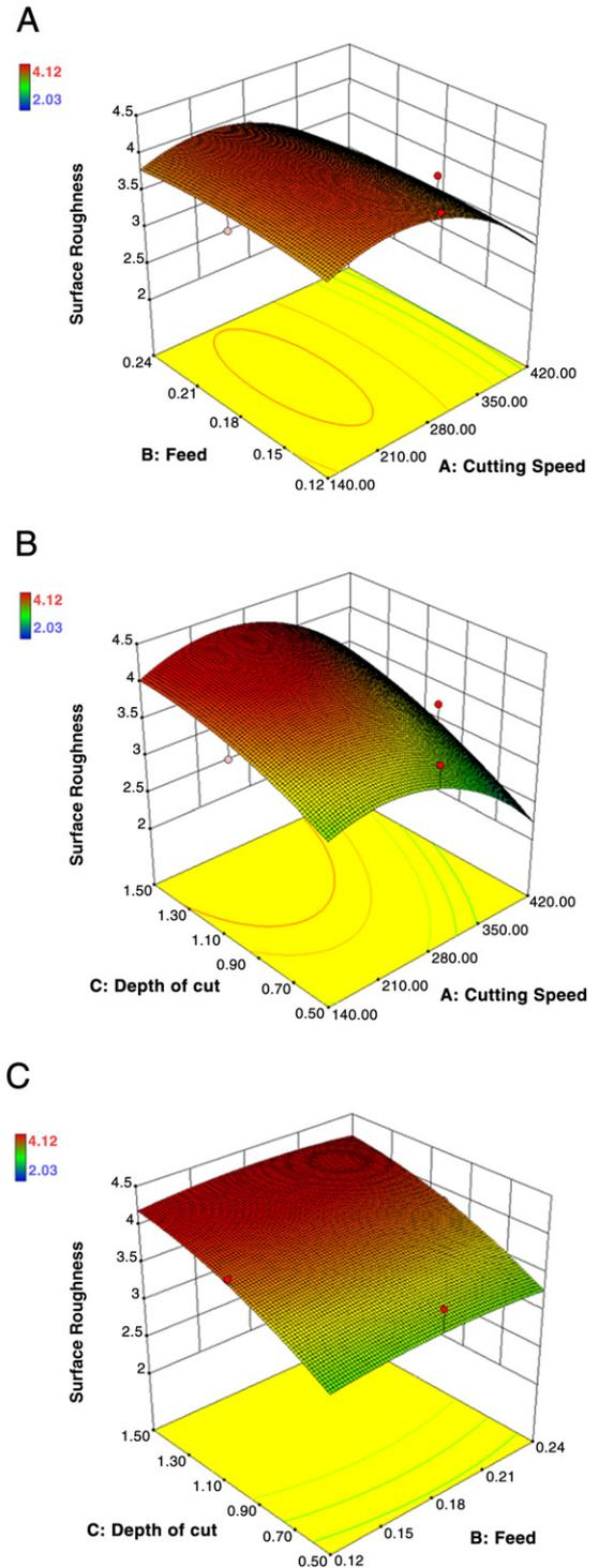
Fig. 4. (A). Interaction effects of surface roughness with feed & cutting speed. (B). Interaction effects of surface roughness with depth of cut & cutting speed. (C). Interaction effects of surface roughness with depth of cut & feed rate.
