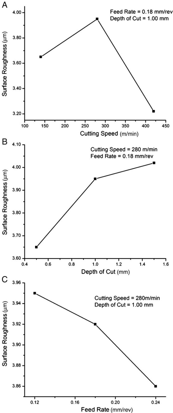
Fig. 3. (A). Direct effects of cutting speed on surface roughness. (B). Direct effects of depth of cut on surface roughness. (C). Direct effects of feed rate on surface roughness.
