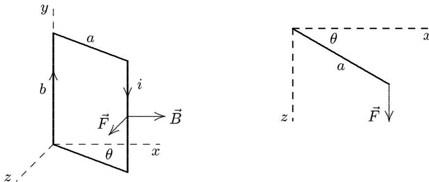
The situation is shown in the left diagram above. The  $y$  axis is along the hinge and the magnetic field is in the positive  $x$  direction. A torque around the hinge is associated with the wire opposite the hinge and not with the other wires. The force on this wire is in the positive  $z$  direction and has magnitude  $F = NibB$ , where  $N$  is the number of turns.
