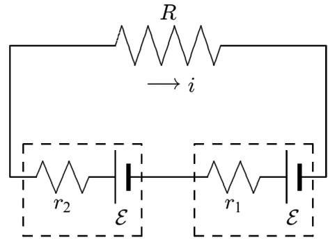
Now assume that the potential difference across battery 2 is zero and carry out the same analysis. You should find  $R = r_2 - r_1$ . Since  $r_1 > r_2$  and  $R$  must be positive, this situation is not possible. Only the potential difference across the battery with the larger internal resistance can be made to vanish with the proper choice of  $R$ .
