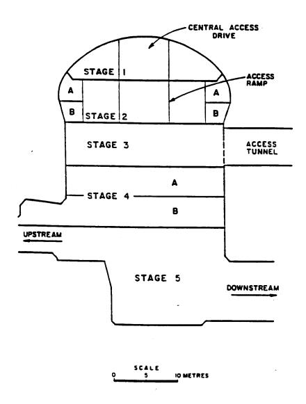
Figure 5: Cavern profile and excavation stages.
