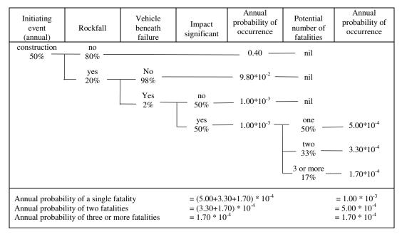
Figure 13: Event tree for a hypothetical example in which construction activities on the Argillite Cut are carried out for a period of six months while the highway is kept open.
