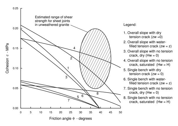
Figure 9: Comparison of the shear strength mobilised by failure under various conditions with the estimated shear strength available on sheet joints in unweathered granite.
