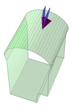
Figure 11: Perspective view of roof wedge in the Rig Grande cavern roof. The size of this wedge has been defined by setting the trace length of the 50/345 joint to 6 m. Eight 10 m long 50 tonne capacity grouted anchors give a factor of safety of 1.6.
