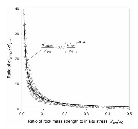
Figure 8: Relationship for the calculation of  $\sigma_{3\text{max}}$  for equivalent Mohr-Coulomb and Hoek-Brown parameters for tunnels.
