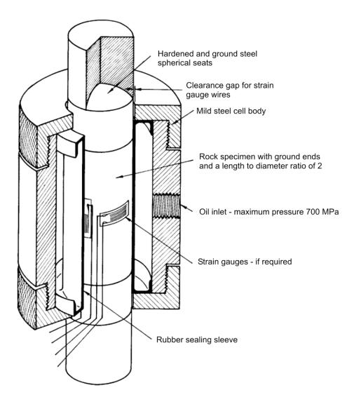
Figure 1: Cut-away view of a triaxial cell for testing rock specimens.
