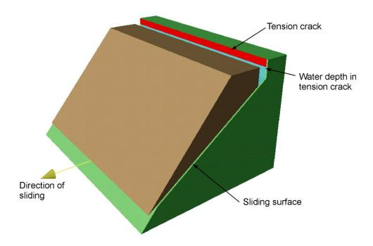
Figure 3: RocPlane model of Sau Mau Ping slope.
