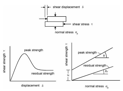
Figure 1: Shear testing of discontinuities
