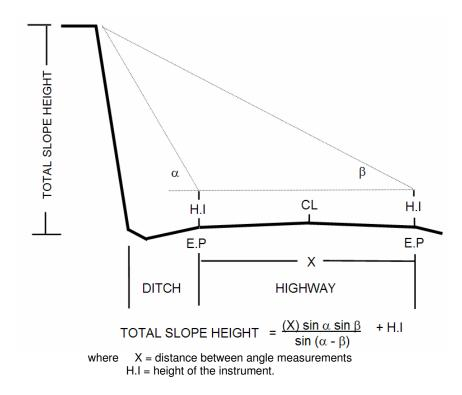
Figure 10: Measurement of slope height.
