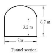
A tunnel is to be excavated in this rock mass and the cross-section of the ramp is given in the sketch. The axis of the tunnel is inclined at 15° to the horizontal or, to use the terminology associated with structural geology analysis, the tunnel axis plunges at 15°. In the portion of the tunnel under consideration in this example, the axis runs due north-south or the trend of the axis is 180°.
