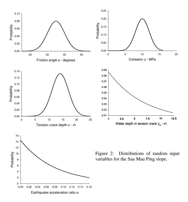
Figure 2 illustrates the plots of the probability distribution functions of the random input variables. It is worth discussing each of the plots in detail to demonstrate the reasoning behind the choice of the probability distribution functions.
