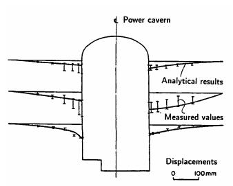
Figure 9: Comparison between calculated and measured displacements along six extensometers installed in the sidewalls of the Mingtan power cavern.
