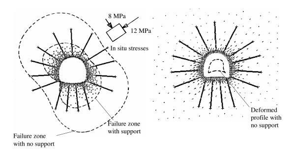
Figure 29: Results of a numerical analysis of the failure of the rock mass surrounding the Yacambu-Quibor tunnel when excavated in graphitic phyllite at a depth of about 600 m below surface.
