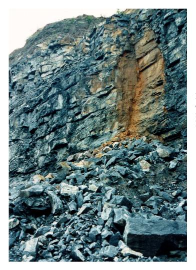
Figure 31: Structurally controlled failure in the face of a steep bench in a heavily jointed rock mass.
