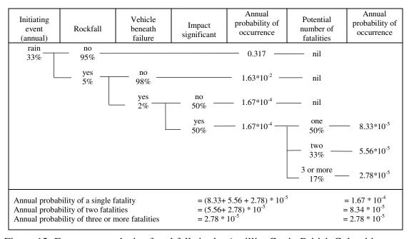
Figure 12: Event tree analysis of rockfalls in the Argillite Cut in British Columbia.
