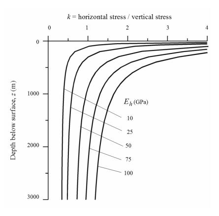
Figure 2: Ratio of horizontal to vertical stress for different deformation moduli based upon Sheorey's equation. (After Sheorey 1994).
