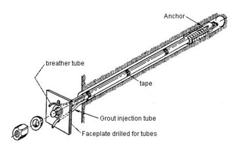
Figure 2: Mechanically anchored rockbolts of the type used on the Rio Grande project. These bolts were tensioned to 70% of their yield load upon installation and then, at a later stage, were re-tensioned and fully grouted.
