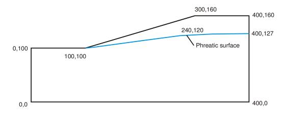
Figure 14: Slope and phreatic surface geometry for a homogeneous slope.
