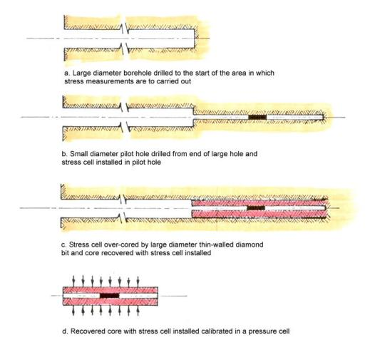
Figure 11: Typical sequence of over-coring stress measurements.
