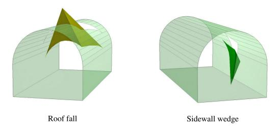
Unless steps are taken to support these loose wedges, the stability of the back and walls of the opening may deteriorate rapidly. Each wedge, which is allowed to fall or slide, will cause a reduction in the restraint and the interlocking of the rock mass and this, in turn, will allow other wedges to fall. This failure process will continue until natural arching in the rock mass prevents further unravelling or until the opening is full of fallen material.
