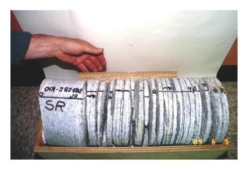
Figure 10: Disking of a 150 mm core of granite as a result of high in situ stresses.
