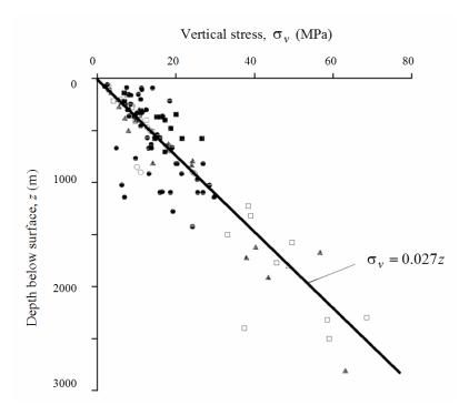
Figure 1: Vertical stress measurements from mining and civil engineering projects around the world. (After Brown and Hoek 1978).
