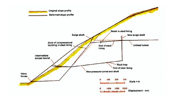
Figure 3: Cross-section through a section of the Wahleach power tunnel showing the original tunnel alignment and the location of the replacement conduit. The dashed line is the approximate location of a gradational boundary between loosened, fractured and weathered rock and more intact rock. Down-slope movement currently being monitored is well above this boundary.
