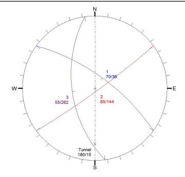
Figure 1: An equal area lower hemisphere plot of great circles representing the average dip and dip directions of three discontinuity sets in a rock mass. Also shown, as a chain dotted line, is the trend of the axis of a tunnel excavated in this rock mass. The tunnel plunge is marked with a red cross.
