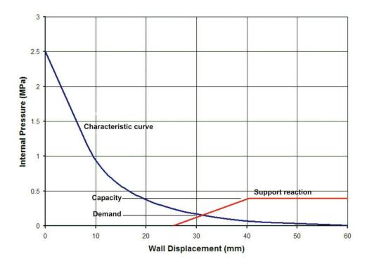
Figure 17: Rock support interaction diagram for a 10 m diameter tunnel subjected to a uniform in situ stress of 2.5 MPa.
