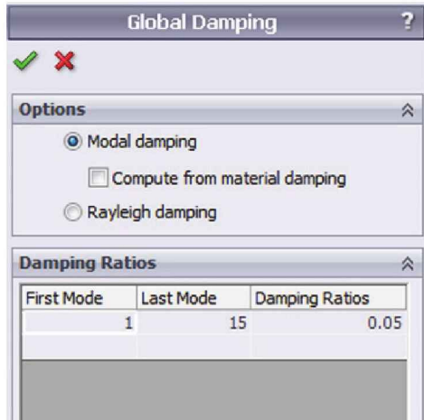
Figure 12-11: Modal damping definition for the three studies simulating a Frequency Sweep.
