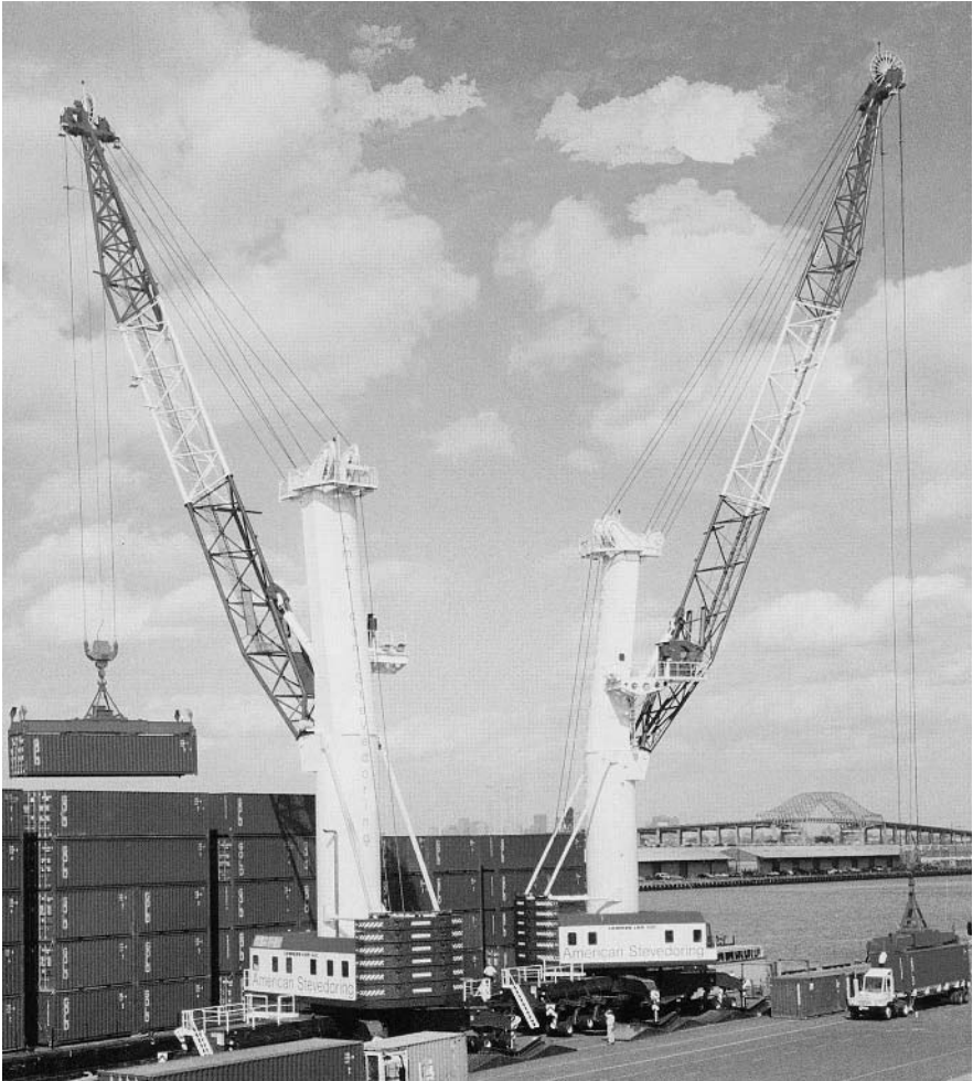
Fig. 1.1.6 100 t mobile 'all-purpose' crane
