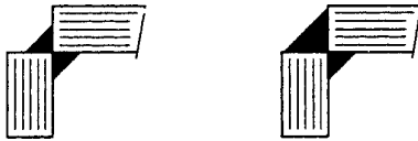
Fig. 7.2.3 Reduction of the sensitivity to lamellar tearing
