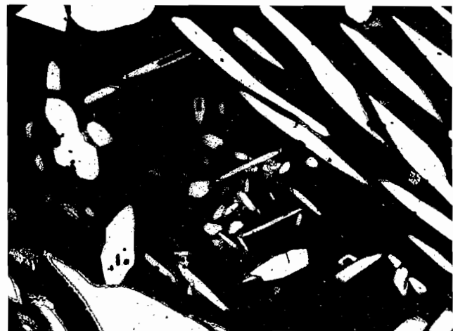
Figure 5. Microstructure of the Material Specimen Number 21 Material 9.4460, Hardened, HB about 550. a) Scale 100:1; b) Scale 500:1.
