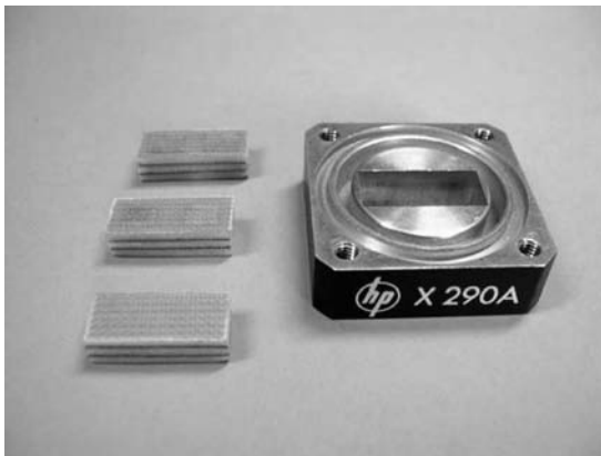
Figure 3.16. Samples for waveguide simulator measurements.
