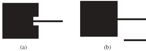
Figure 3.5. Patches with attached stubs. (a) Indented line, (b) folded line.
