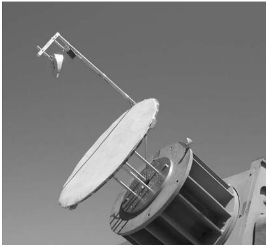
Figure 6.12. 0.75-m Cassegrain offset-fed X/Ka dual-band reflectarray mounted on antenna range pedestal.
