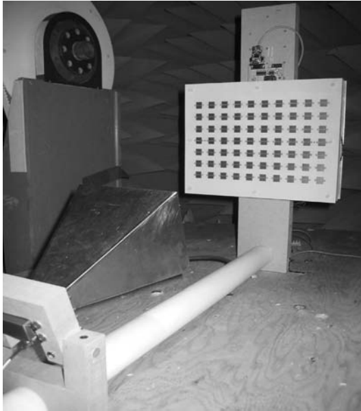
Figure 7.65. Photo of the 70-element C-band beam scanning reflectarray with tunable varactor diodes. (Courtesy of Dr. Sean Hum and Prof. Michal Okoniewski of Univ. of Calgary, Canada.)
