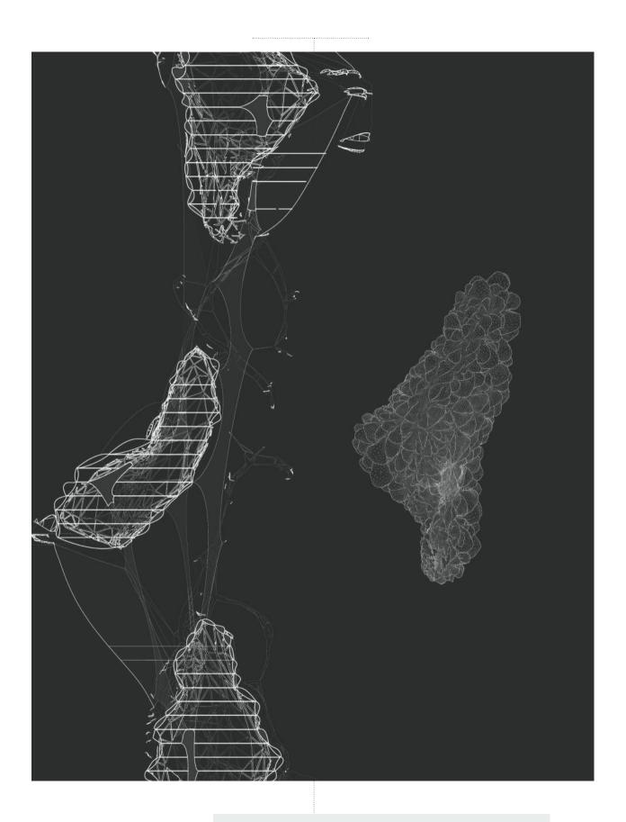
Peter Macapia, Section Study, GrTplgy Tower, 2008 Section study of a primary tetrahedral structure in which a secondary and compressive variable structural system is coupled with a cable tensile system and ETFE membrane.
