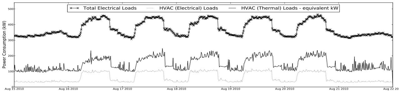
Figure 1: Power consumption breakdown for our building. The HVAC electrical load is between 25% to 33% of the total electrical load. The HVAC thermal load, as expressed in kW equivalent of cooling, is also significant.
