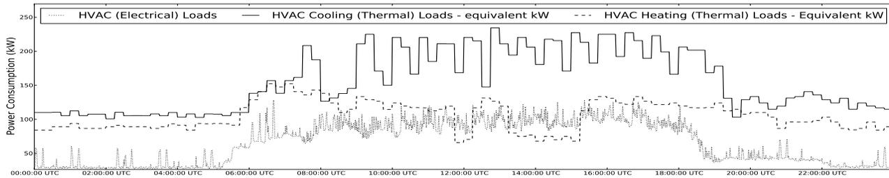
Figure 10: The energy consumption of HVAC during our second test day. We graph both electrical loads and thermal loads (as equivalent kW). The HVAC-electrical savings compared to baseline shown in Figure 8 are 9.54% while the HVAC-thermal savings are 12.85% and 11.51% for cooling and heating loads respectively.
