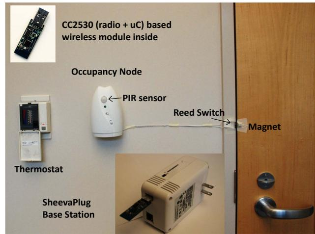
Figure 4: Occupancy node deployed on the wall of an office. The reed switch, PIR sensor and our CC2530 based radio module inside the occupancy node are also shown.
