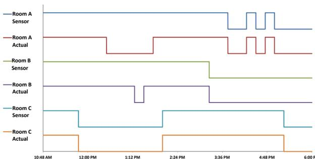
Figure 6: Accuracy test of three representative rooms over seven hours.
