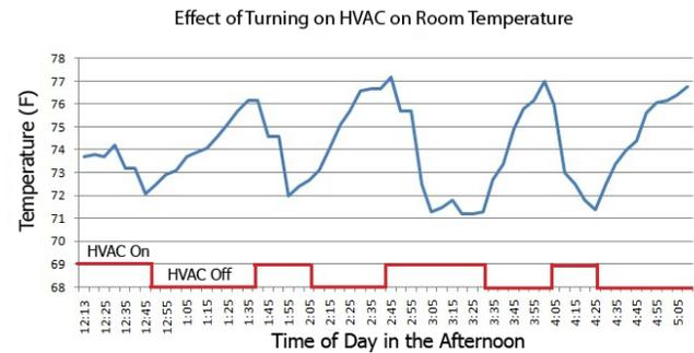
Figure 11: Effect of actuating HVAC for an IT-heavy room facing towards the sun during a warm day.
