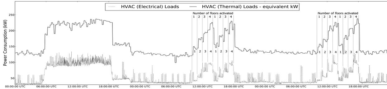
Figure 2: HVAC power consumption - Friday Oct 22nd to Sunday Oct 24th. The first day is a regular day (Friday) that shows the HVAC as is without any duty-cycling and all floors are ON as normal. The next day is Saturday when we turn on one floor at a time – 1 floor HVAC on (10AM – 11AM), then 2 floors (11AM – Noon), 3 floors (12PM – 1PM), 4 floors (1PM – 2PM), then turn all floors off and repeat from 2PM to 6PM. We repeat the same experiment on Sunday.
