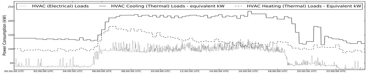
Figure 8: The energy consumption of HVAC during our baseline day. We show HVAC electrical loads as well as the HVAC thermal loads for both cooling and heating (as equivalent kW).
