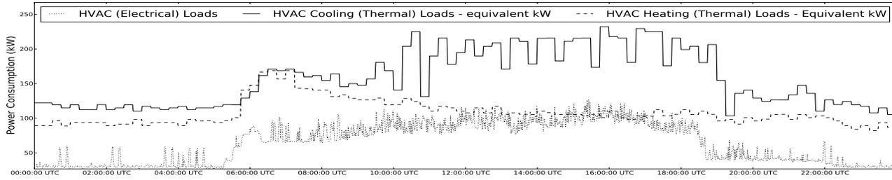
Figure 9: The energy consumption of HVAC during our first test day. We graph both electrical loads and thermal loads (as equivalent kW). The HVAC-electrical savings compared to baseline shown in Figure 8 are 11.59% while the HVAC-thermal savings are 12.41% and 9.59% for cooling and heating loads respectively.
