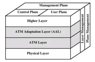
The reference model for ATM approximately maps to the three lowest layers of the ISO-OSI reference model: network layer, data link layer, and physical layer.
