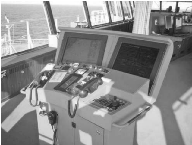
FIGURE 9.11 New bridge wing console, adapted to work when berthing. (Design by Wallenius Marine AB/Furuno Finland. Photograph used with permission.)
