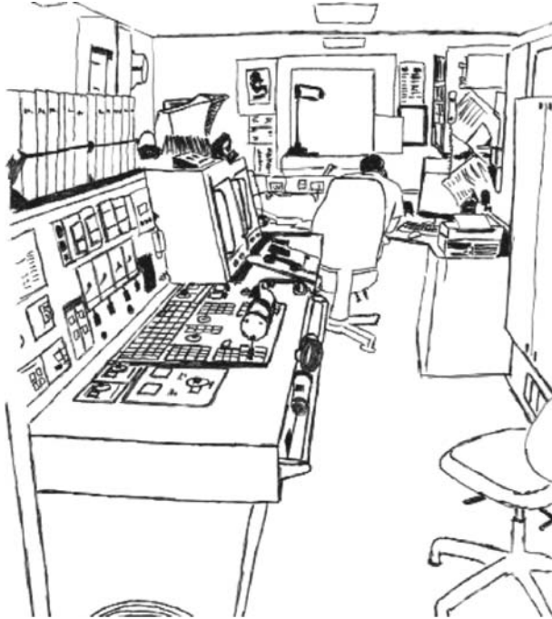
FIGURE 9.20 A narrow desk in the ECR which is in a corner. This leaves the engineer with his back to the operating panels and the alarm system. (Drawing by E. Jacobson from a photograph. With permission.)
