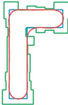
Figure 7: An example of Optical Proximity Correction . The green mask produces the red structure after photolithographic imaging (illustration from Wikipedia).
