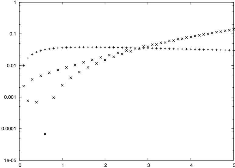
Figure 17.3 Comparison of relative absolute errors (17.2) for the centered scheme (17.1) ( $\times$ 's) and the explicit Euler scheme (16.26) ( $+$ 's) for solving  $u' = -u^2$ .
