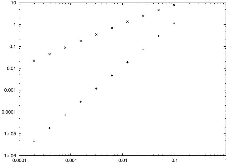
Figure 17.1 Absolute error in computing  $e^\pi \approx 23.141$  by the explicit Euler method (16.26) ( $\times$ 's) and by the centered scheme (17.1) ( $+$ 's). The horizontal axis is  $\Delta t$ , and the vertical axis is the absolute error at  $T = 1$ .
