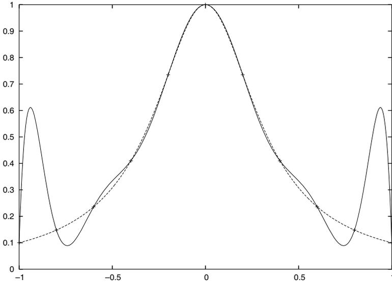
Figure 10.2 The Runge function  $r_3$  (dashed line) and its Lagrange interpolant for 11 equally spaced interpolation points on the interval  $[-1, 1]$ . The “+” signs indicate the interpolation data.
