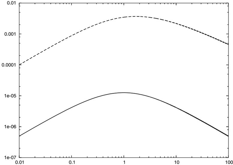
Figure 17.6 Relative absolute errors (17.2) for the explicit Euler scheme (16.26) (upper curve) and the improved Euler scheme (17.6) (lower curve) for solving  $u' = -u^2$ , using  $\Delta t = 0.01$ . The horizontal axis is time.
