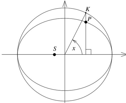
Figure 2.1 The notation for Kepler's equation. The sun is at  $S$  (one of the foci of the elliptical orbit), the planet is at  $P$ , and the point  $K$  lies on the indicated circle that encloses the ellipse of the orbit; the horizontal coordinates of  $P$  and  $K$  are the same, by definition. The angle  $x$  is between the principal axis of the ellipse and the point  $K$ .
