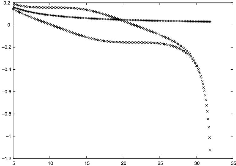
Figure 17.4 Comparison of values  $u_n$  computed via the centered scheme (17.1) ( $\times$ 's) with those computed via the explicit Euler scheme (16.26) ( $+$ 's) for solving  $u' = -u^2$ , integrated until  $T = 32$ .
