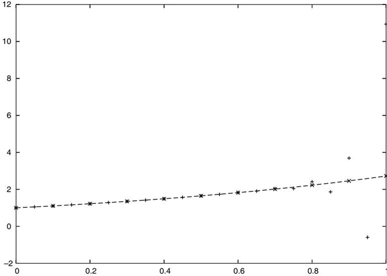
Figure 17.5 Result of using (17.5) to solve  $u' = u$  on  $[0, 1]$  with two different values for the time step  $\Delta t = 0.1$  ( $\times$ 's) and  $\Delta t = 0.05$  ( $+$ 's). The horizontal axis is  $t$ , and the vertical axis is the value of  $u$ .
