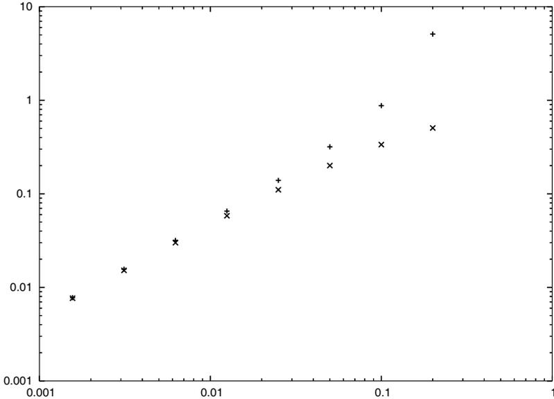
Figure 16.2 Relative errors in computing  $e^\pi$  by the explicit Euler method (16.26) ( $\times$ 's) and the implicit Euler method (16.27) (+'s). The horizontal axis is  $\Delta t$ , and the vertical axis is the relative error at  $T = 1$ .
