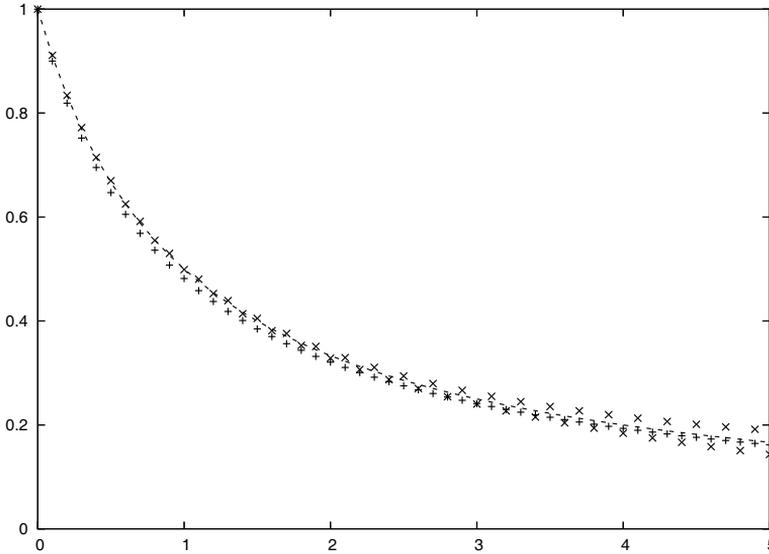
Figure 17.2 Comparison of values  $u_n$  computed via the centered scheme (17.1) ( $\times$ 's) with those computed via the explicit Euler scheme (16.26) ( $+$ 's) for solving  $u' = -u^2$ . The dotted line is the exact solution (16.5).
