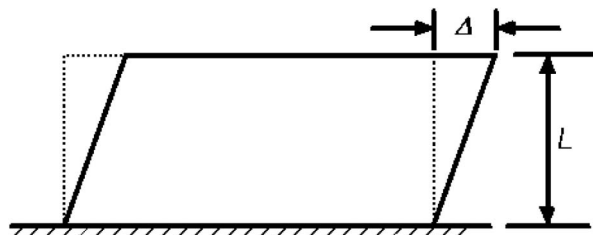
Figure 10-5. Story Drift in Structural Wall Where Shear Dominates Inelastic Response
