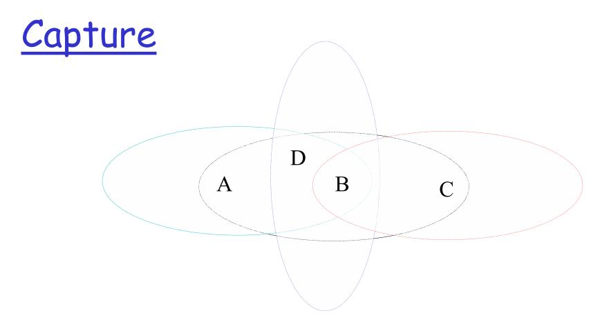
□ Capture is said to occur when a receiver can cleanly receive a transmission from one of two simultaneous transmissions both within its range
