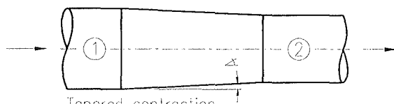
Tapered contraction SP_2 = SP_1 - (VP_2 - VP_1) - L(VP_2 - VP_1)
