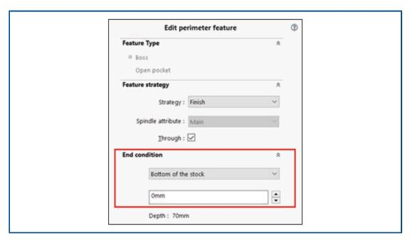
You can store end condition settings for the part perimeter feature in the Technology Database. This data is helpful in automating and maintaining consistency between parts that are similar when programming.
