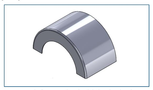
You can create edge flanges on nonlinear (circular) edges of nonplanar faces.
