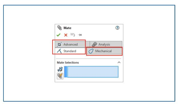
In the Mate PropertyManager, the standard, mechanical, and advanced mate types moved into separate tabs.
