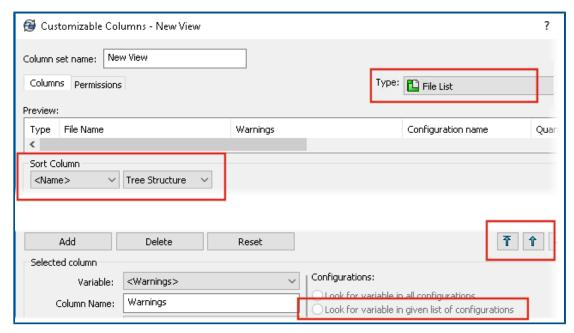
SOLIDWORKS PDM offers flexibility and control for column sets. You can assign multiple column sets to users or groups for all column set types. In SOLIDWORKS PDM File Explorer, you can view the file list based on assigned column sets.
