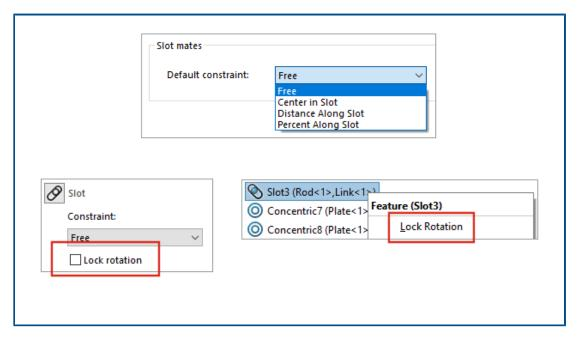
You can specify a default constraint type and lock the rotation for slot mates.
