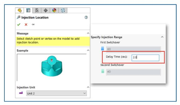
You can specify a delay time between injections of the first and second material for Co-injection, Gas-assist, and Water-assist processes.
