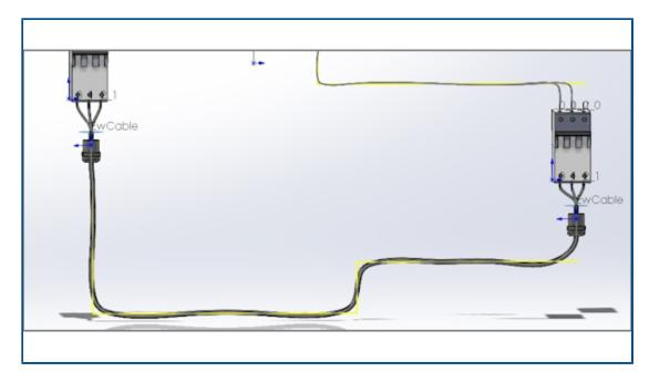
You can route electrical harnesses using splines.
