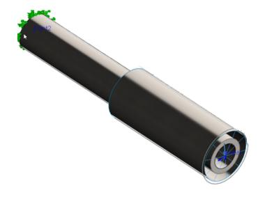
The gap between the two cylinders represents the shell thickness (inner solid body, outer shell body). In reality, the two cylinders are touching with no clearance.
