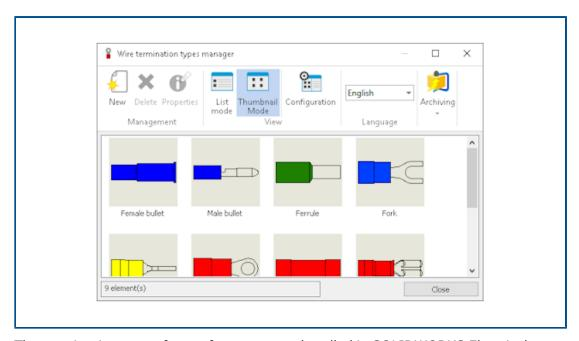
The termination type of manufacturer parts handled in SOLIDWORKS Electrical propagates automatically to the connector properties.
