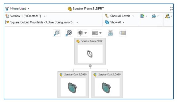
SOLIDWORKS PDM 2021 extends Treehouse view in the Contains tab to the Where Used tab. This helps you to view all the parent relationships of the selected child in a hierarchical and graphical format.
