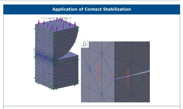
Example of two bodies that have an initial clearance and come into contact under load application. Contact stabilization enables the accurate solution in SOLIDWORKS Simulation 2021.
