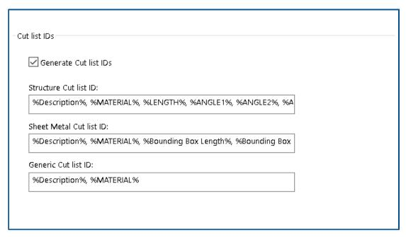
You can generate cut list IDs or unique reference IDs for each cut list in a cut list folder based on the cut list attributes.
