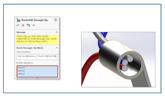
When you want to use clips in a routing assembly, you can select multiple routes simultaneously. You can also define how the cable cores appear inside the clip.
