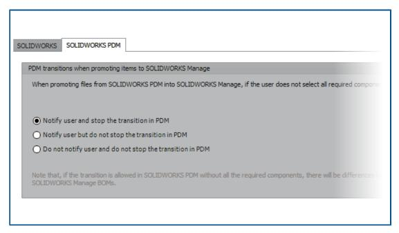
You can select the options that are available to define the handling of missing file references during promotion through SOLIDWORKS PDM state change.
