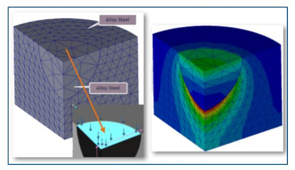
Simulations for linear static studies are more accurate for curved surfaces that come into contact.
