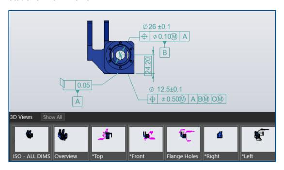
eDrawings displays annotations in the text scale specified for the 3D View in SOLIDWORKS part and assembly files.
