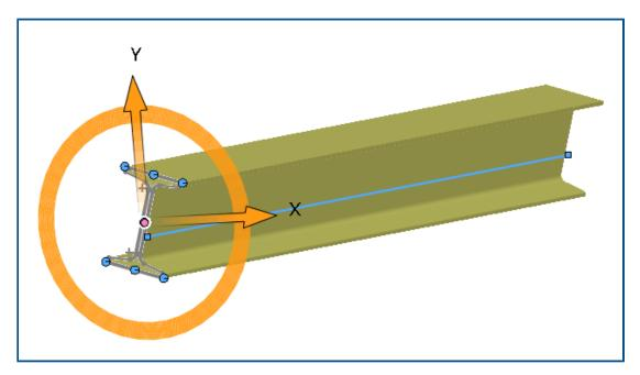
You can interact graphically on screen with the profile of the structural member. When you select the profile, the graphical manipulator appears in the graphics area at the pierce points. You can drag the profile horizontally or vertically, or rotate it to suit your alignment.
