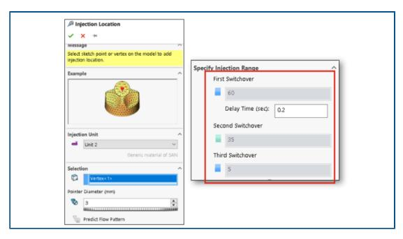
You can simulate an A-B-A sequence of a Co-injection molding process.
