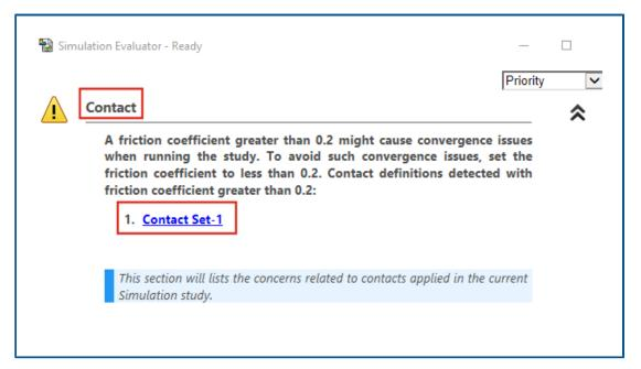
The Simulation Evaluator is enhanced to flag study definitions related to the assigned friction coefficient for contacts and materials for invalid Poisson's ratio values.
