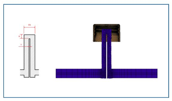
Modeling is improved for baffles and bubblers that are part of cooling system components.
