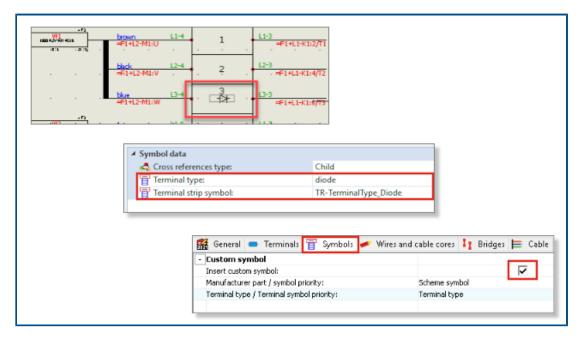
You can associate a specific terminal symbol used in a terminal drawing either to a manufacturer part or to a terminal symbol used in a schematic. This allows you to have a different representation of the terminals in the terminal strip drawing.
