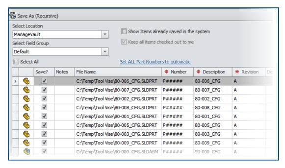
The **Save as (Recursive)** option in the SOLIDWORKS Manage add-in for SOLIDWORKS imports assemblies and references. It also applies the numbering scheme defined in SOLIDWORKS Manage to those assembly structures.
