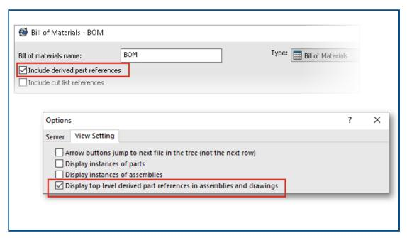
The support for the derived part references is improved and you can view them in the file view tabs and SOLIDWORKS PDM Add-in.
