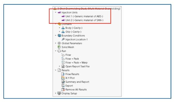
The PlasticsManager tree is redesigned to provide a more streamlined and logical workflow for creating plastics simulation studies. A new node, **Injection Units**, replaces **Injection System**.
