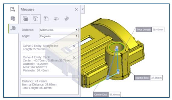
eDrawings Web HTML files support the Move and Measure tools.
