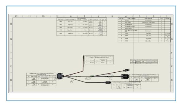
When you generate a flattened route, the tables are inserted in specific locations.
