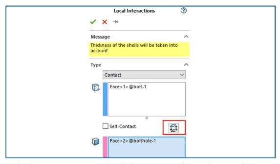
For local interactions, you can switch the geometry selections between the source and target sets to resolve convergence issues. When you are working with complex geometries that have multiple faces, switching the geometry entities between the source and target sets with the **Swap interaction faces** tool saves you time.
