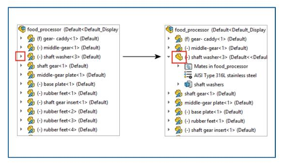
For assemblies opened in lightweight mode, top-level components and subassemblies resolve automatically when you click be to expand the item in the FeatureManager design tree. Components in subassemblies remain in lightweight mode until you expand them.
