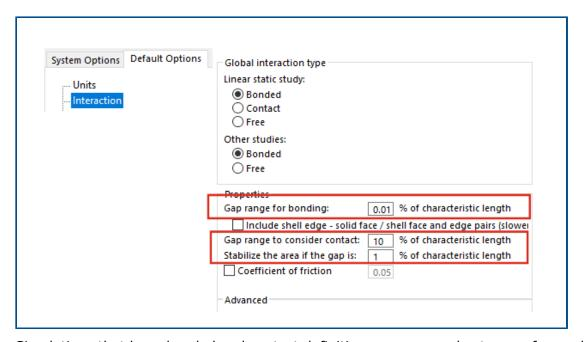
Simulations that have bonded and contact definitions are more robust, even for models with slightly imperfect geometries. Algorithms that detect clearances between geometries
