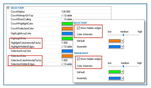
You can control the visibility of hidden edges when you select or highlight elements. You can define the color and intensity used to display hidden edges.
