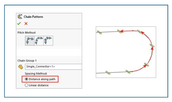
You can define spacing between chain pattern instances as a measure along a path for **Distance** and **Distance Linkage** chain patterns.
