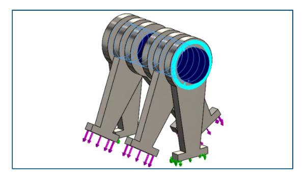
Listing pin connector loads at the pin joints is more accurate for shear forces and bending moments in the global or a user-defined coordinate system.
