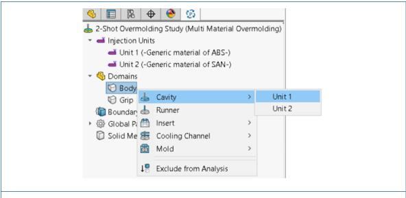
Example of a cavity domain assignment for a two-shot overmolding process. A cavity is associated with injection unit 1. Two injection units are defined.
