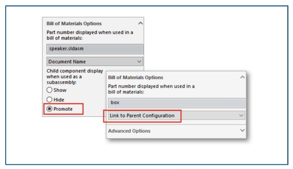
SOLIDWORKS PDM uses the Bill of Materials component display settings that are specified in SOLIDWORKS.
