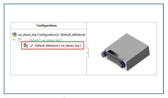
When you use the **Silhouette** method for defeaturing, you can create a configuration from a defeatured assembly. In the assembly, you can switch between the defeatured configuration and the full model.
