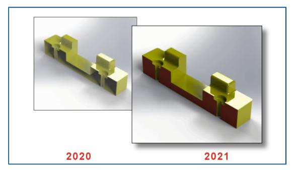
When you create a section view, you can cap the geometry that the cut plane slices.
