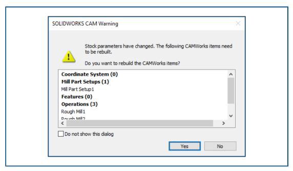
In the **Mill** module, when you modify stock parameters after generating features, options, or toolpaths, a warning lets you rebuild data for entities affected by the change. These entities may include coordinate systems, mill part setups, features, and operations.
