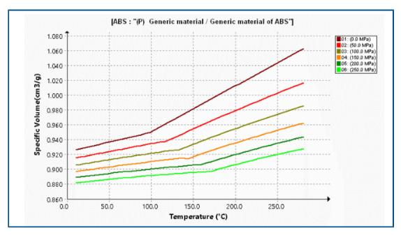
There are several enhancements to the display of Viscosity and Pressure-Volume-Temperature (PVT) plots.
