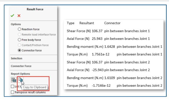
You can copy tabular simulation results displayed inside PropertyManagers to the clipboard and paste the copied data from the clipboard into a Microsoft® Excel® or Word document. You can copy reaction forces, free body forces, contact/friction forces, connector forces, and probed results.
