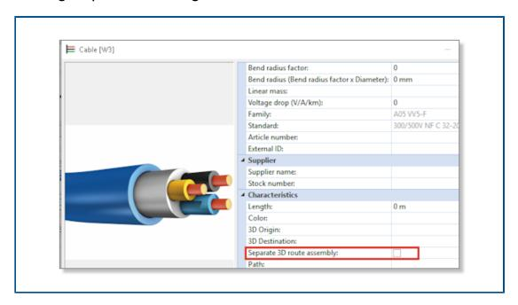
You can generate a separate routing assembly of cables. Specify the **Separate 3D route assembly** option in the cable properties. You can select one, several, or all cables to route.
