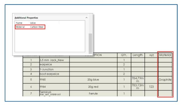
You can display more properties that are assigned to connectors and wires in BOMs.
