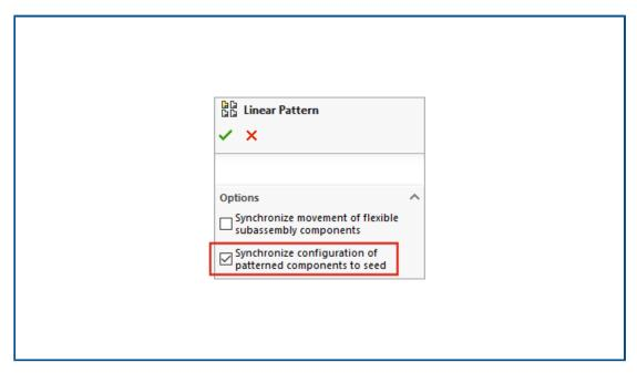
You can use **Synchronize configuration of patterned components to seed** to block changes to the configuration of patterned instances.
