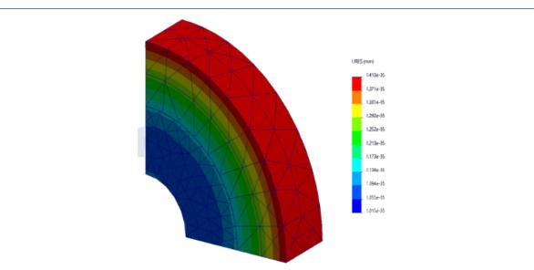
With the integration of geometry corrections, the deformation contour plot is accurate (SOLIDWORKS Simulation 2021).
