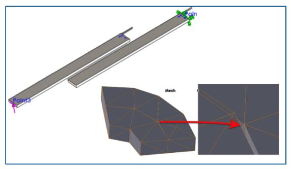
The accuracy of results for static, frequency, and buckling studies is improved for geometries that have bonded interactions. Improved algorithms that mesh bodies independently drive this improvement.
