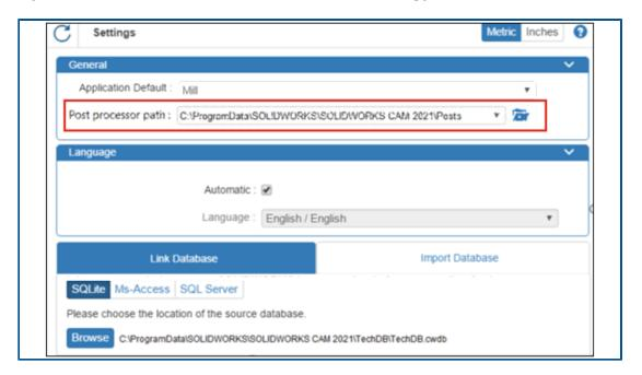
In the Settings tab of the Technology Database, you can specify a folder location for post processors associated with a Mill or Turning machine.
