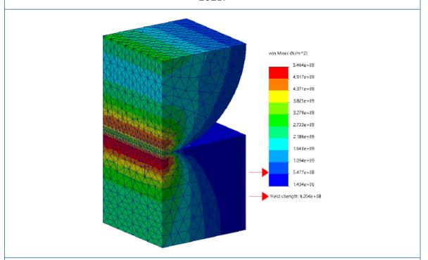
Accurate stress plot results with the enablement of contact stabilization in SOLIDWORKS Simulation 2021.
