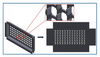
Flat patterns use efficient algorithms to identify bend connections. This reduces the time to flatten complex sheet metal bodies with many flanges by about 20-25 times.
