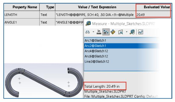
You can calculate the correct cut list length of a weldment member in the cut list properties.
