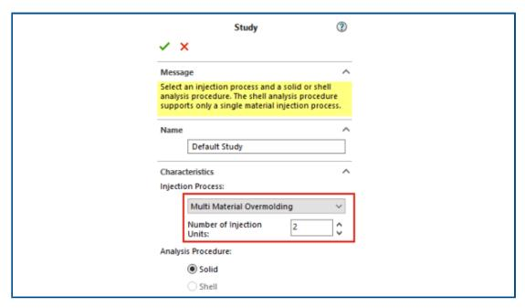
You can inject two to six different polymer materials within the same cycle.
