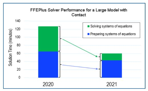
The solution time of linear static studies with many surface-to-suface contact elements is improved. The **Intel Direct Sparse** solver can handle linear static and nonlinear studies with more than 4 million equations.
