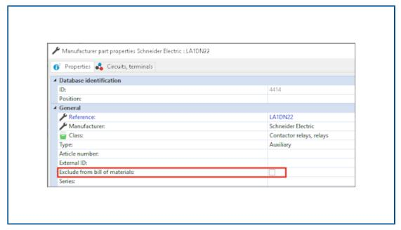
You can use the **Exclude from bill of materials** property in the **Manufacturer part properties** dialog box to show or hide components in a BOM. The property propagates into assemblies and 3D parts.
