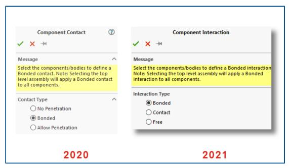
User interface terms related to contact and mesh are updated to match conventional industry terminology. The term Interaction is introduced to describe the type of behavior between components during a simulation (bonded, contact, or free).
