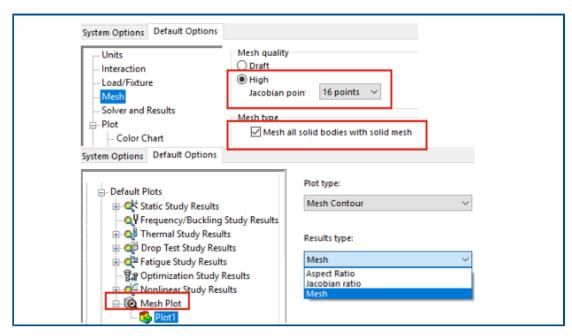
The default mesh settings for new studies facilitate mesh assignments for most models. Enhancements for mesh settings include:
