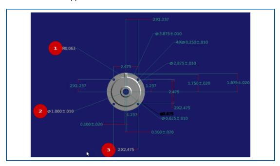
You can open SOLIDWORKS parts with 3D annotations in SOLIDWORKS Inspection Standalone to create inspection documents.
