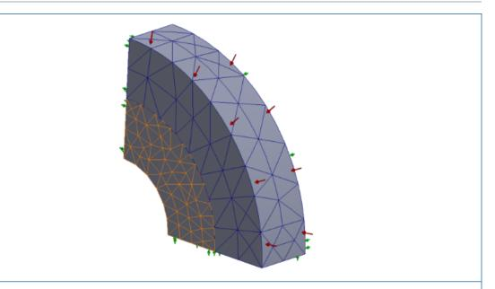
Two cylindrical bodies come into contact under a pressure load. The bodies mesh independently. The inner body has a draft-quality mesh with a higher mesh density. The outer body has a high-quality mesh with a lower mesh density.
