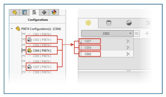
You can specify configurations of a SOLIDWORKS part or assembly model to be available when you open the model in SOLIDWORKS Visualize.
