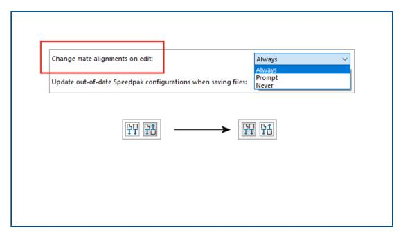
When you flip the alignment of a mate, the edited mate flips.
