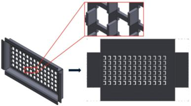
Assembly features can propagate to individual components even if there are multiple instances of the same part in the assembly. Sheet metal parts created in SOLIDWORKS 2013 and later did not support this functionality.
