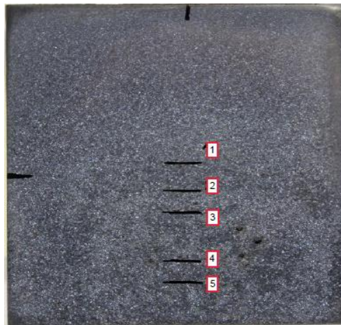
Figure 3.23 Micro etched billet sample 3490L1
