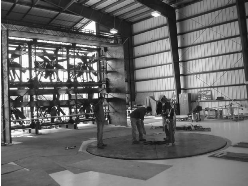
Figure 13.3.6. Six-fan wall of wind, Florida International University (courtesy of Drs. A. Gan Chowdhury and G. Bitsuamlak).
