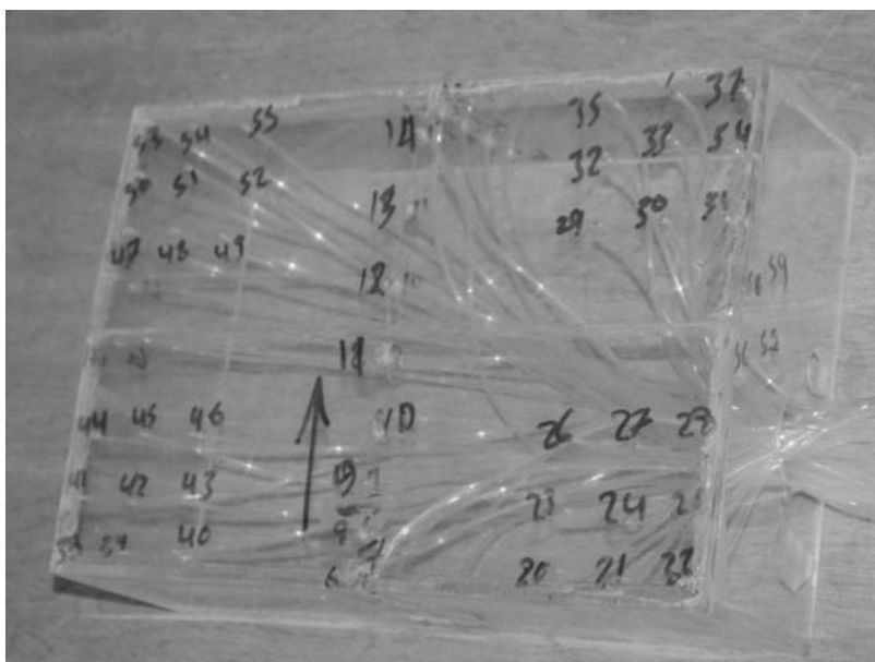
Figure 13.3.3. Pressure taps and tubes installed on a small-scale test building (courtesy of Dr. Aly Mousaad Aly Sayed Ahmed, Alexandria University, Egypt).
