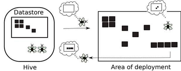
**Figure 2. The hive-drone data model in action. Drones are dispatched with blank scratchpads. As they execute a behavior, they populate their scratchpad. On return to the hive, the scratchpad is appended to the Datastore.**
