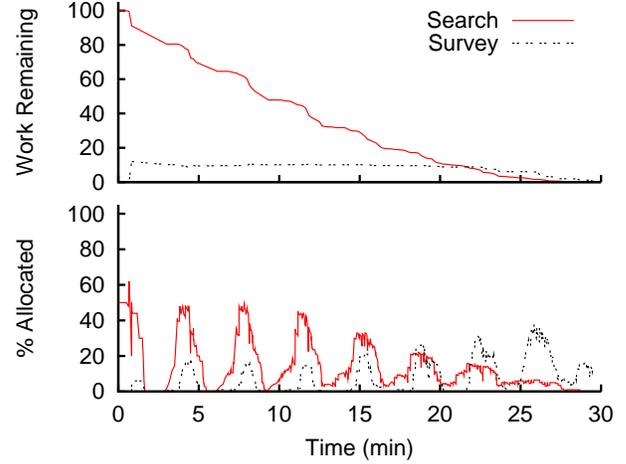
**Figure 6. Karma allocates drones to behaviors according to the estimated amount of work to be done and the measured progress rate of each behavior per region. Remaining work is the sum of remaining progress across all regions.**
