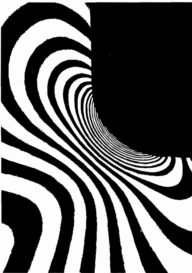
Figure 15. Close-up of T-root Stress Concentration [9].
