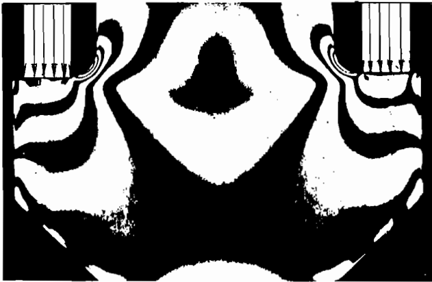
Figure 14. Stress Concentration in Fillet of T-root [3].
