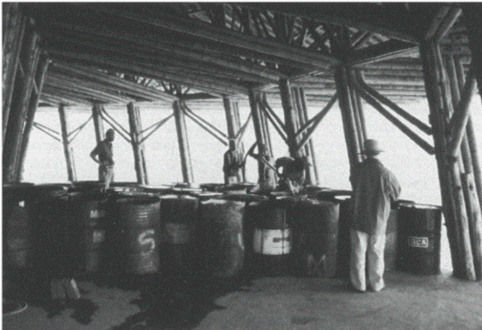
Figure 7.39 Gallery test mass using water ballast.
