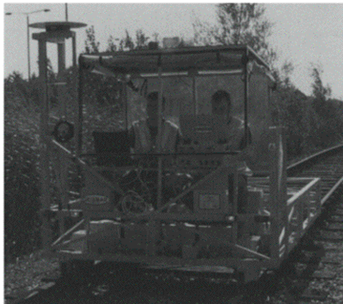
Figure 5.13 Track monitoring vehicle.
