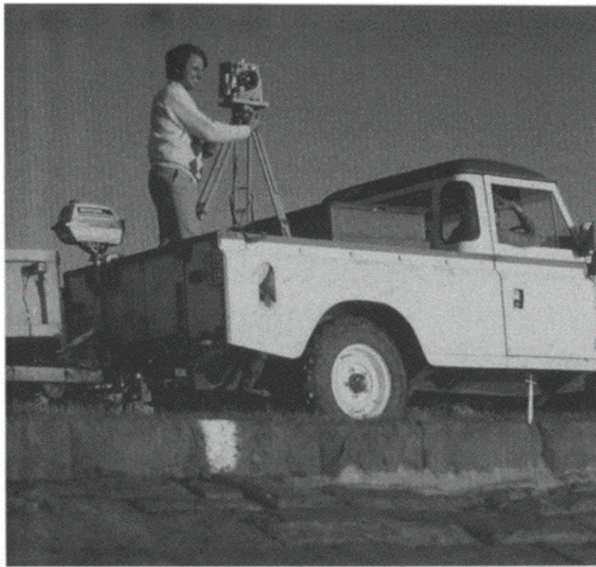
Figure 4.6 UMK mounted in Land Rover to photograph reservoir lining from above.
