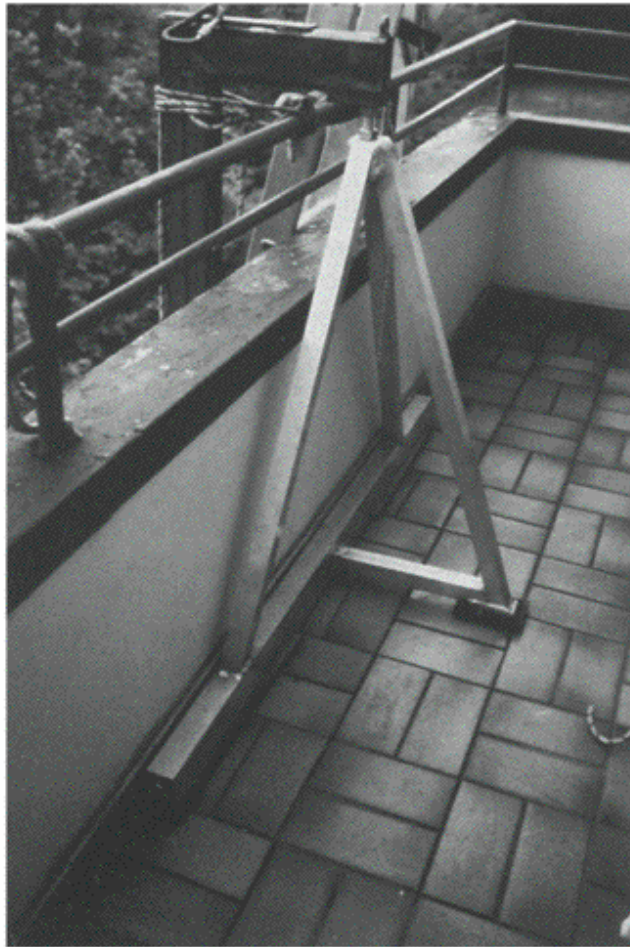
Figure 7.13 Load hook and trestle.
