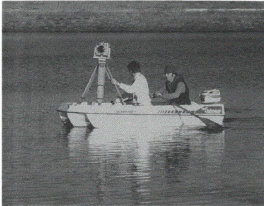
Figure 4.5 UMK camera in small dinghy to photograph reservoir lining.
