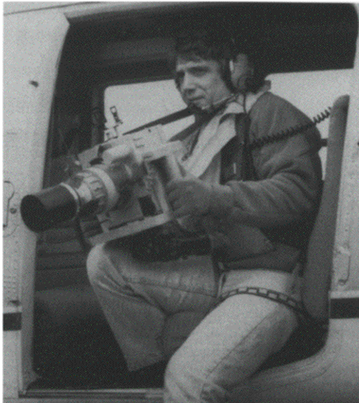
Figure 4.10 300mm focal length Zeiss UMK camera in specially constructed hand-held mount for photography from a helicopter.
