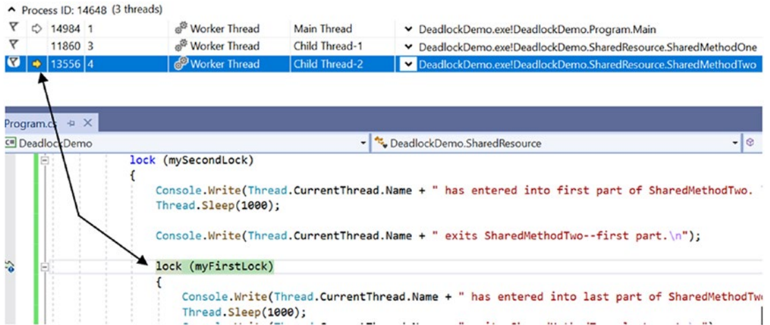
Figure 5-6. Child Thread-2 window in deadlocked state
