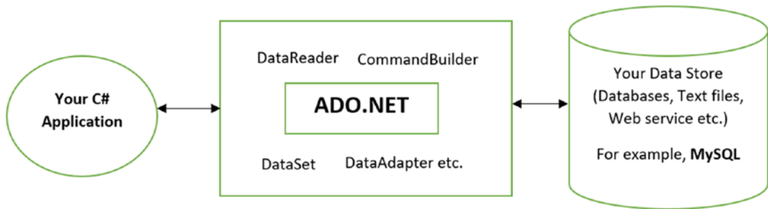
Figure 7-1. Connecting a C# application to a database through ADO.NET
