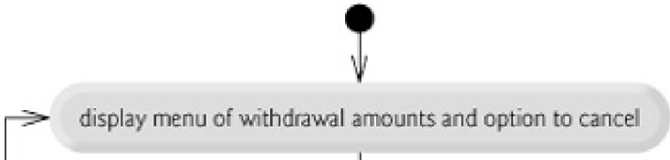
Fig. 5.22. Activity diagram for a Withdrawal transaction.
