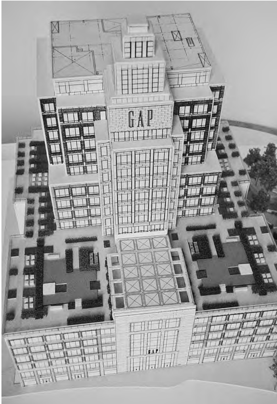
FIGURE 8-4 Study models help to understand scale and explore ways of mitigating the impacts of wind, sun, shade, and orientation.
