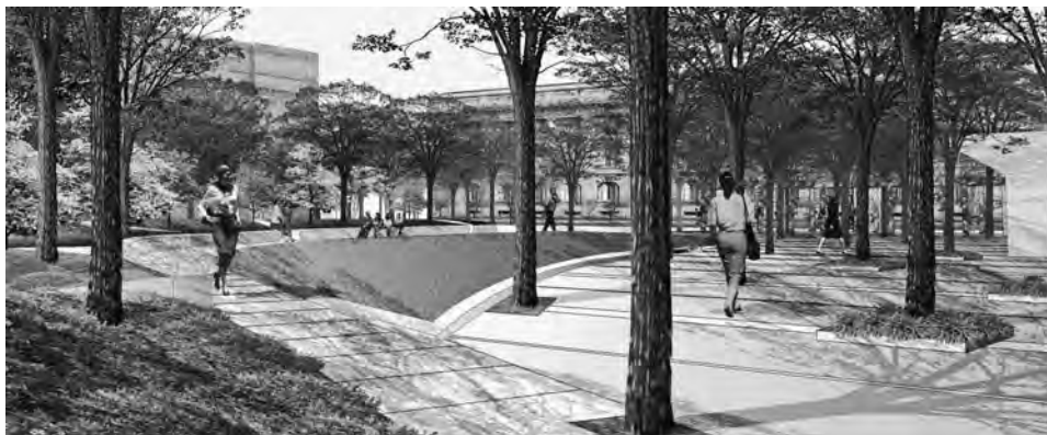
FIGURE 4-21 Perspective of proposed design illustrating location of trees and sculptured earth mounds that help to buffer winds off Lake Erie.
