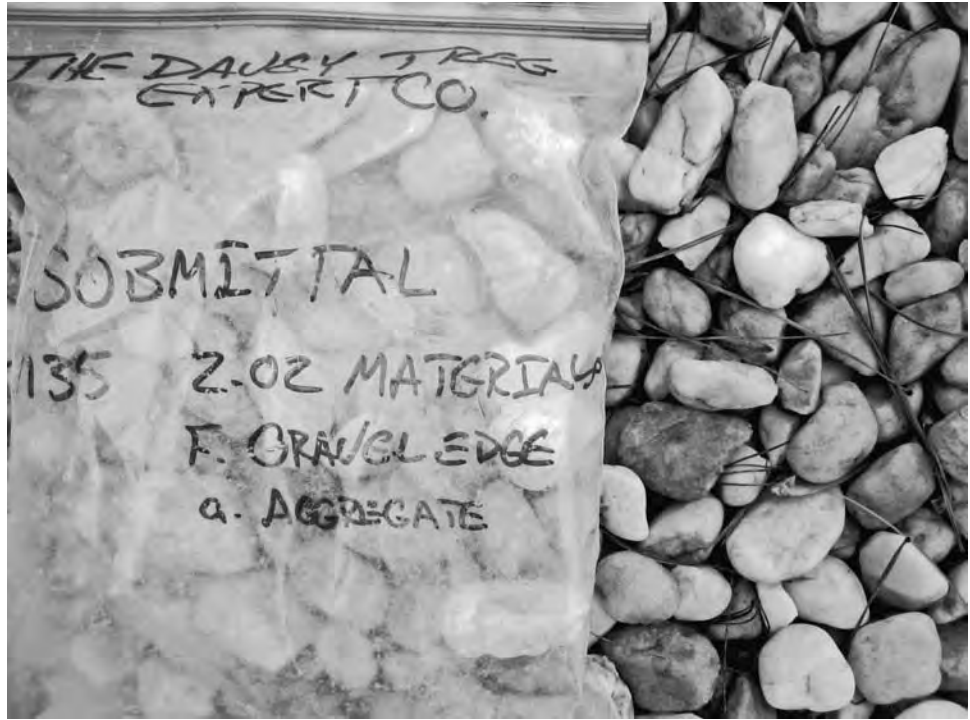
FIGURE 8-43 Submittals for all components of green roof systems should require samples of materials. Here the aggregate used for the gravel edge required around drains and the perimeter of plantings is submitted for approval.
