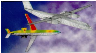
Hybrid mesh and pressure contours on the surface of an aircraft
