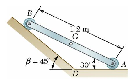
The extremities of a 1.2 m rod weighing 25 kg can move freely and with no friction along two straight tracks. The rod is released with no velocity from the position shown.
