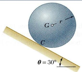
A sphere of weight W is released with no initial velocity and rolls without slipping on the incline.
