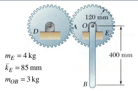
The portion AOB of the mechanism is actuated by gear D and at the instant shown has a clockwise angular velocity of 8 rad/s and a counterclockwise angular acceleration of 40 rad/s<sup>2</sup>.
