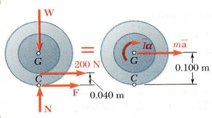
$$\bar{I} = m\bar{k}^2 = (50 \text{kg})(0.70 \text{m})^2$$
