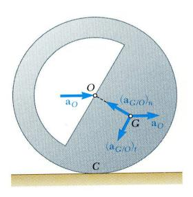
For a balanced disk constrained to roll without sliding,
