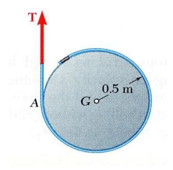
A cord is wrapped around a homogeneous disk of mass 15 kg. The cord is pulled upwards with a force T = 180 N.
