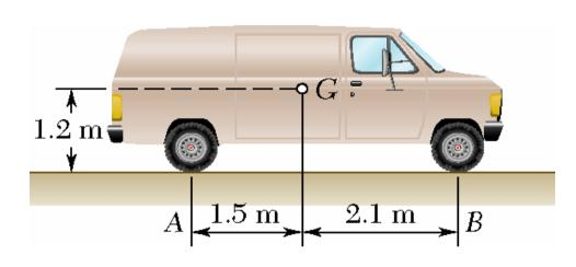
At a forward speed of 10 m/s, the truck brakes were applied, causing the wheels to stop rotating. It was observed that the truck to skidded to a stop in 6 m.
