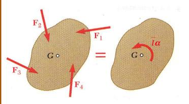
• Motion of a rigid body in plane motion is completely defined by the resultant and moment resultant about *G* of the external forces.
