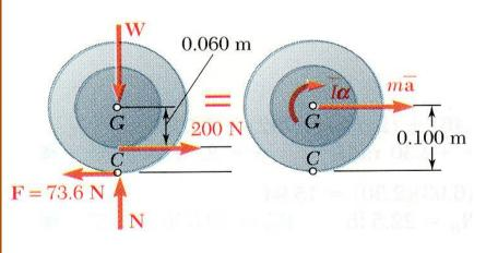
• Compare the required tangential reaction to the maximum possible friction force.
