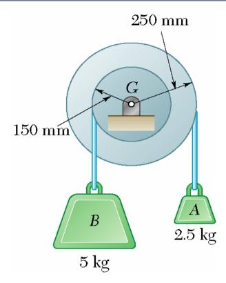
A pulley weighing 6 kg and having a radius of gyration of 200 mm is connected to two blocks as shown.
