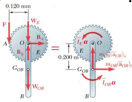
• Solve the three scalar equations derived from the free-body-equation for the tangential force at *A* and the horizontal and vertical components of reaction at *O*.
