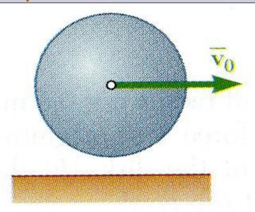
A uniform sphere of mass m and radius r is projected along a rough horizontal surface with a linear velocity  $v_0$ . The coefficient of kinetic friction between the sphere and the surface is  $\mu_k$ .
