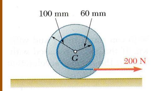
A cord is wrapped around the inner hub of a wheel and pulled horizontally with a force of 200 N. The wheel has a mass of 50 kg and a radius of gyration of 70 mm. Knowing  $\mu_s = 0.20$  and  $\mu_k = 0.15$ , determine the acceleration of G and the angular acceleration of the wheel.
