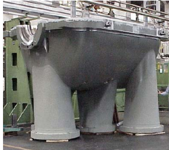
Figure 37. Large Horizontally Split Casing.
