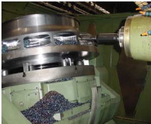
Figure 36. Five Axis Milling of Centrifugal Impeller.
