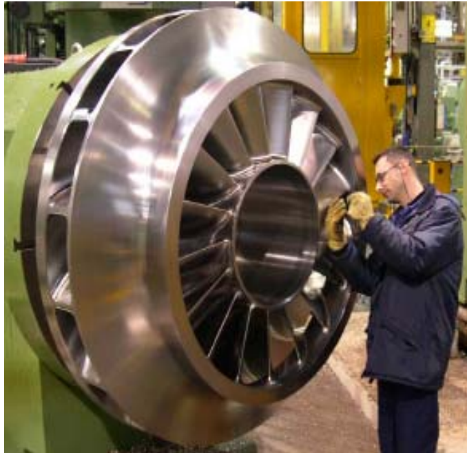
Figure 35. Large 1750 mm (5. 7ft) Diameter 3D Centrifugal Impeller.
