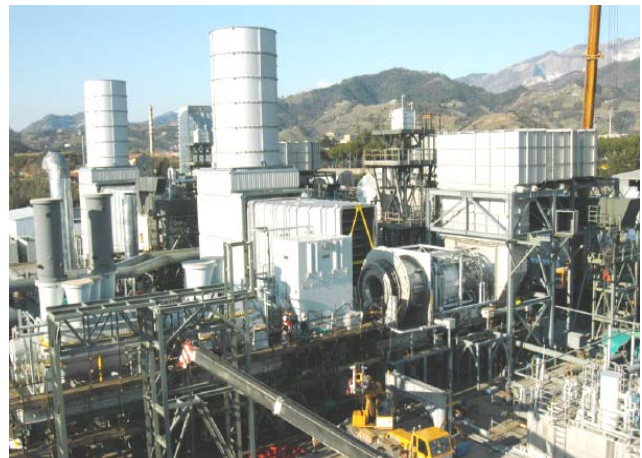
Figure 81. Frame 7—LNG Compressor String Test Setup.
