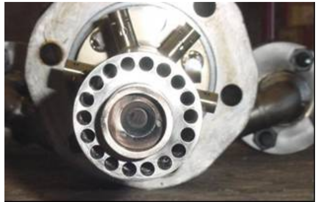
Figure 29. Secondary Fuel Nozzles.
