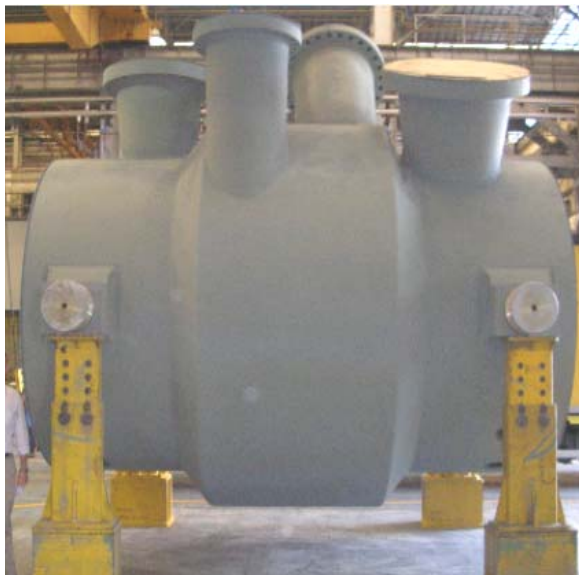
Figure 45. Large Barrel type LNG Compressor.
