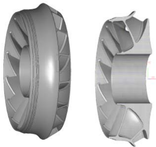
Figure 56. Mixed Flow Impeller.
