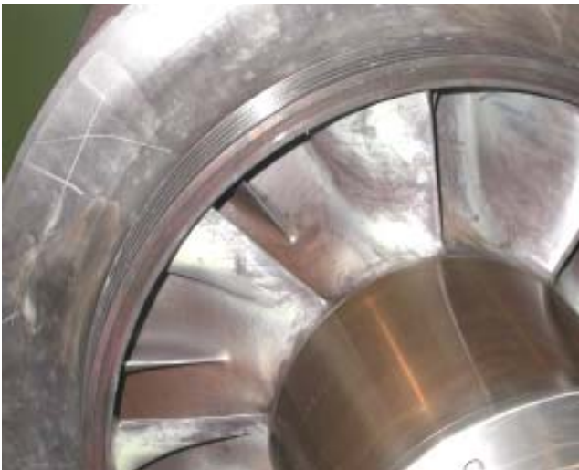
Figure 57. Centrifugal Compressor with Splitter Vanes.
