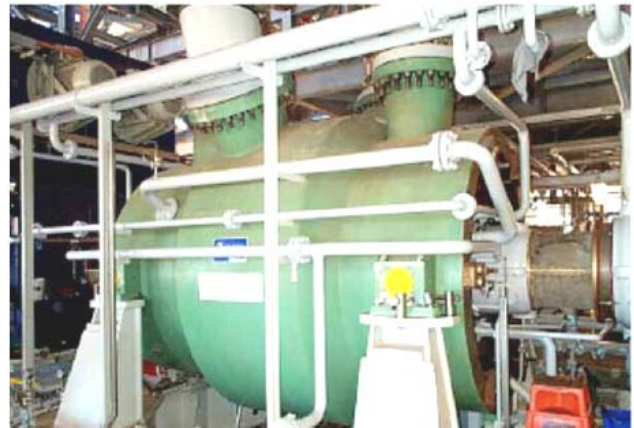
Figure 49. Back-to-Back Barrel Compressor.
