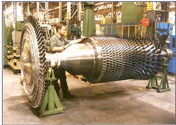
Figure 11. Frame 5D High Pressure Rotor (Axial Compressor and High Pressure Turbine).
