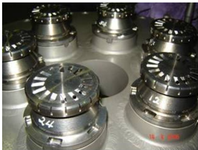
Figure 28. Primary Fuel Nozzles.
