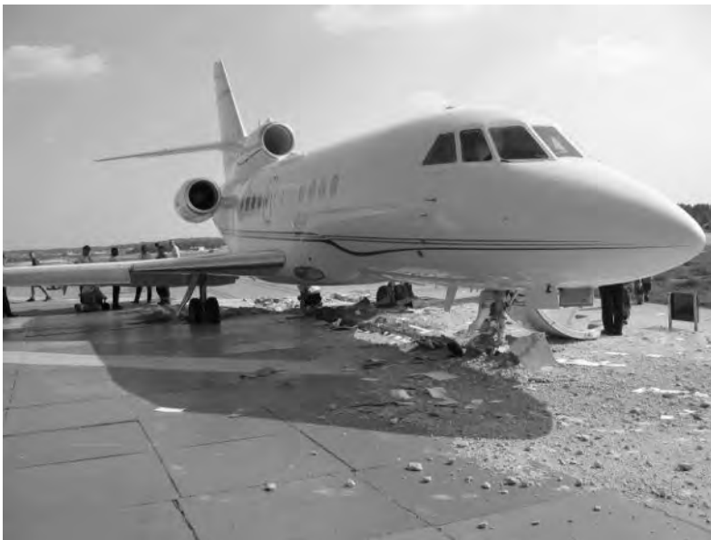
Figure 5-4 The Dassault Falcon 900 business jet successfully arrested by the ZODIAC-ESCO EMAS system at Greenville Downtown airport on 17 Jul 2006 (Courtesy ESCO ZODIAC, photo: David J. Heald, C.M.)
