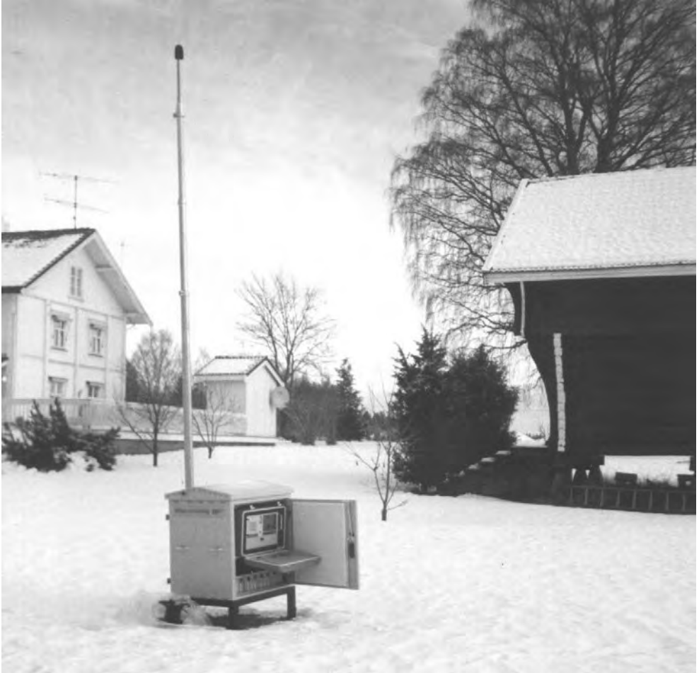
Figure 20-4 Terminal for a permanent aircraft noise monitoring Environmental Sound Analyzer NOR 121 with a multi-spectral analyze and audio recording from a sound events of fly-over, NORSONIC AS Norway, with control unit and post-processing software TOPSONIC Ltd. Germany (Photo: Courtesy NORSONIC AS)
