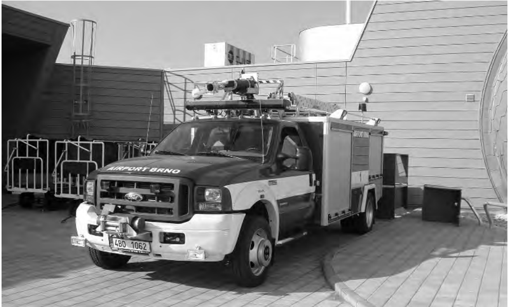
Figure 19-4 Rapid intervention vehicles must reach the accident location first (Photo: A. Kazda)
