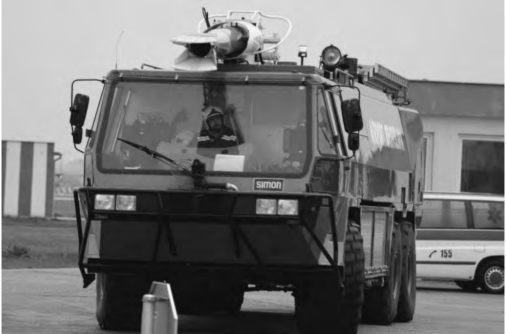
Figure 19-5 Main vehicle carry water for the foam preparation
