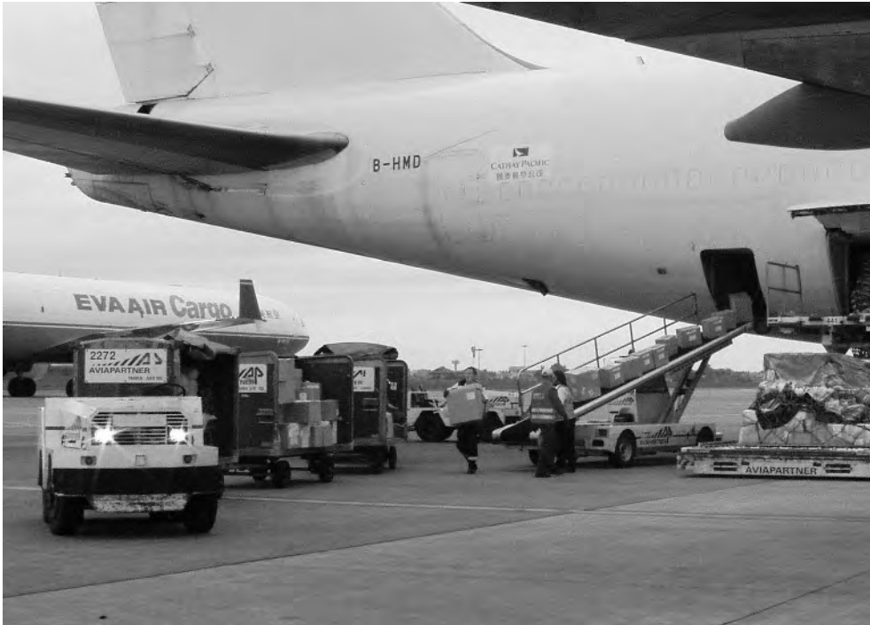
Figure 11-4 Bulk loading cargo into a belly hold (Photo: A. Kazda)
