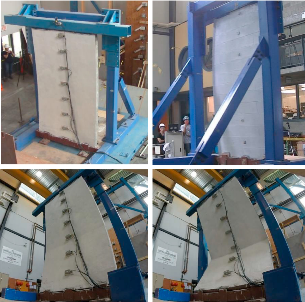
Fig. 5. Different views of the single sided wall at extreme deformations at 200% intensity of the 2011 Tohoku Earthquake of Japan
