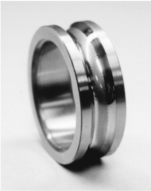
Figure 4-51. Bearing “fluting” caused by bearing currents (Courtesy of ABB Inc.)
