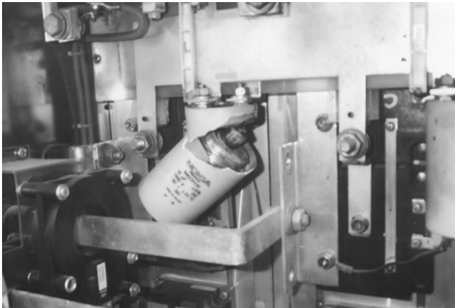
Figure 7-6. Capacitor failure (Courtesy of ABB Inc.)
