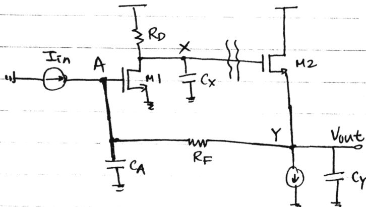
Breaking the loop at node X as shown by {{}} and replacing each end by the impedance each sees, we get the next circuit :
