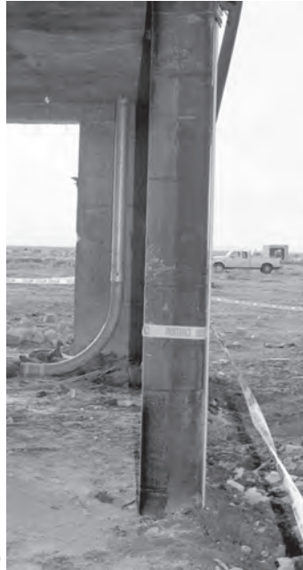
Figure 17.2 Depiction of results from full-scale blast testing of retrofitted and unretrofitted RC columns (Photo courtesy of DTRA): (a) Unretrofitted column (Test 1), (b) Steel jacket column (Test 2), (c) FRP wrapped column (Test 3).
