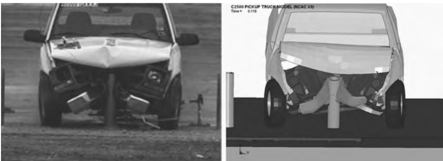
Figure 12.7 Front View of Impact versus Analysis Result (Compliments of Applied Research Associates, Inc.)
