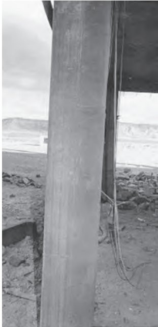
Figure 17.2 Depiction of results from full-scale blast testing of retrofitted and unretrofitted RC columns (Photo courtesy of DTRA): (a) Unretrofitted column (Test 1), (b) Steel jacket column (Test 2), (c) FRP wrapped column (Test 3).
