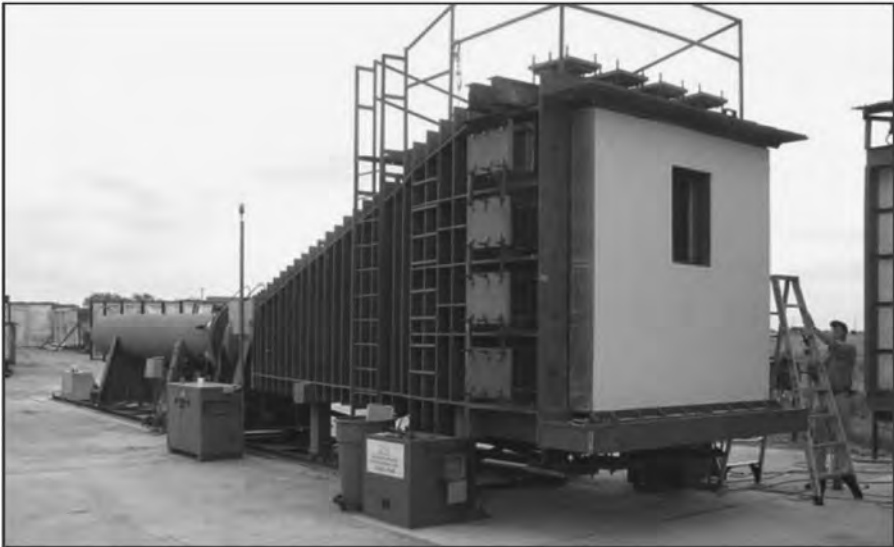
Figure 5.5 Shock Tube Blast Simulator
