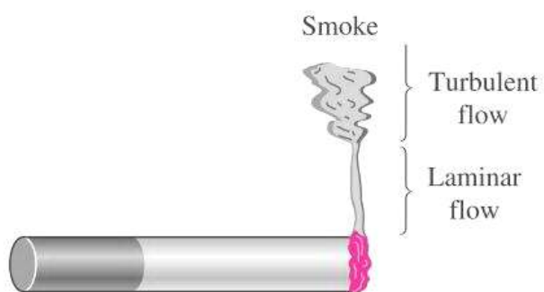
Laminar and turbulent flow regimes of cigarette smoke.
